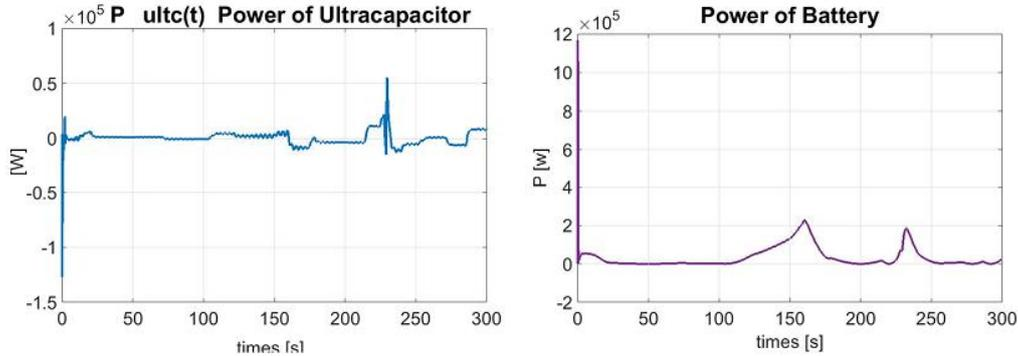
Figure 4.10: Output power of battery and supercapacitor
