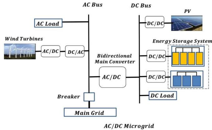
Figure 2.4: Hybrid AC/DC MicroGrid System
