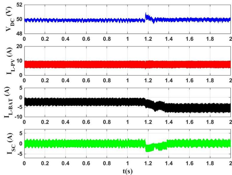
Figure 6.18: Dynamic Response during decreasing load with battery charging
