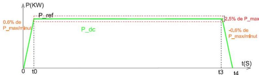
Figure 1.2: Power Profile to be provided for the grid
