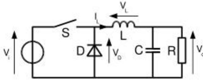
Figure 2.24: Functional circuit of a buck converter
