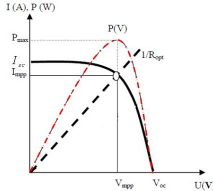
Figure 3.2: Solar cell characteristics
