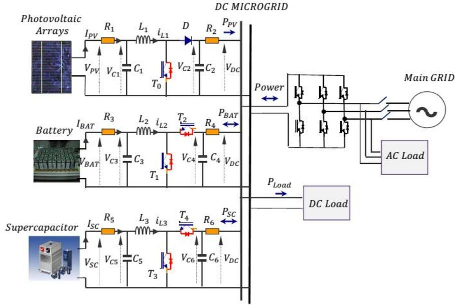
Figure 4.2: DCMicrogrid Configuration
