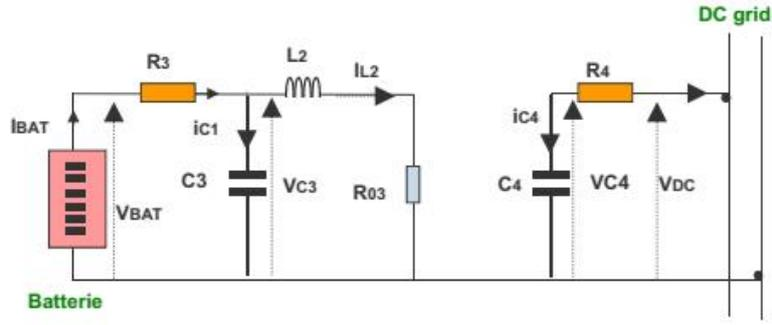
Figure 3.24: The equivalent circuit in interval  $[0, u_2T]$
