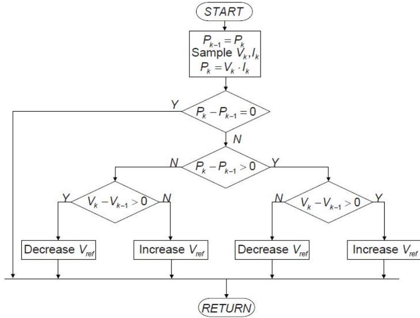
Figure 2.16: Flow chart of P and O algorithm
