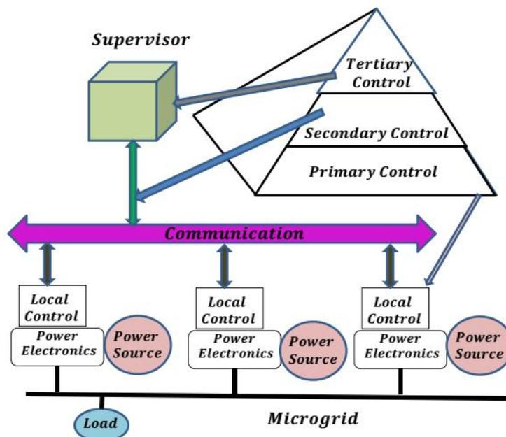
Figure 2.9: Hierarchical control levels
