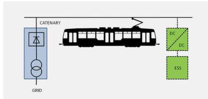
Figure 2.19: braking energy recovery system with storage
