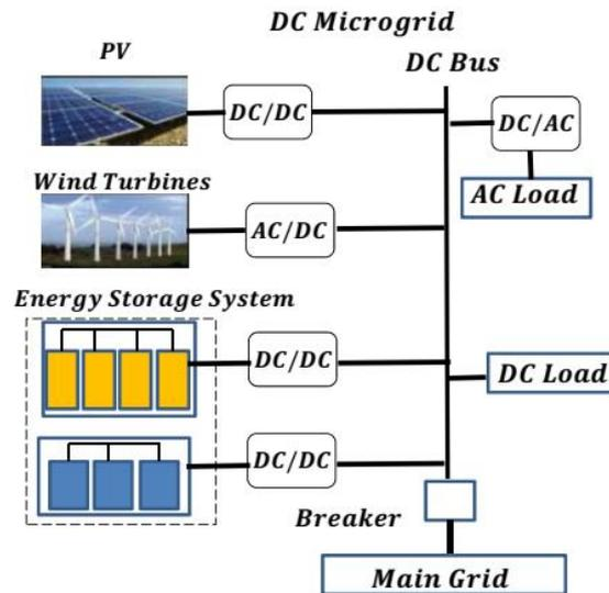
Figure 2.3: DCMicroGrid
