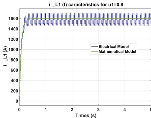
Figure 3.22: Current characteristics for  $u_1 = 0.8$
