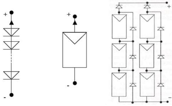
Figure 3.4: PV Array
