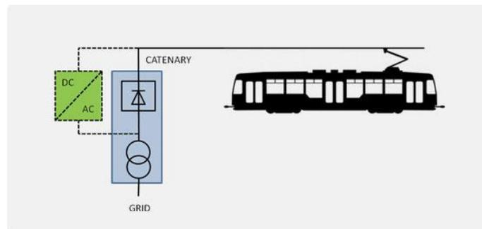
Figure 2.18: braking energy recovery system
