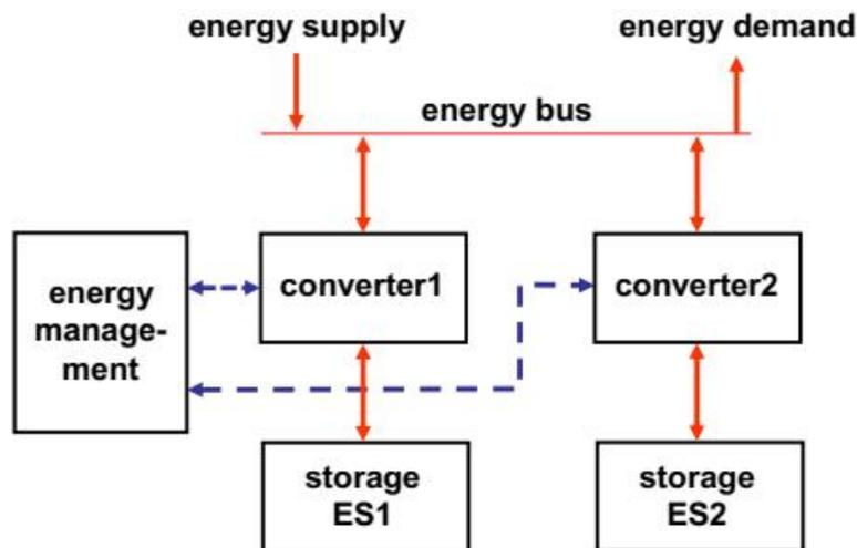
Figure 3.10: Basic structure of a HESS [1].
