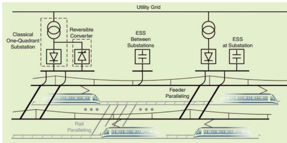
Figure 3.7: Energy-saving techniques in DC-electrified railway systems
