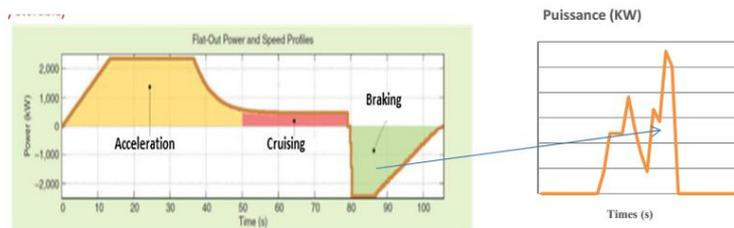
Figure 2.20: Power Profile of braking energy recovery system
