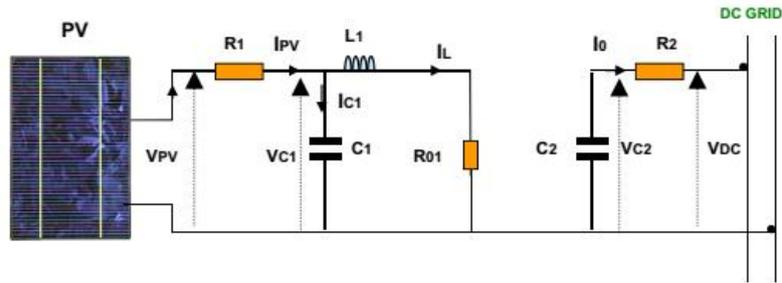
Figure 3.19: The equivalent circuit in interval  $[0, u_1T]$
