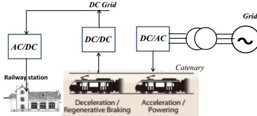
Figure 3.8: Substation Architecture
