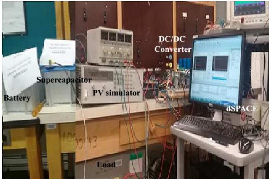
Figure 6.10: Experimental setup
