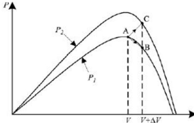
Figure 2.15: Divergence of P and O from MPP
