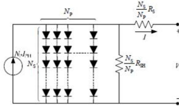
Figure 3.3: Series and parallel connection of solar cells
