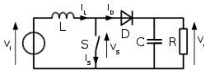
Figure 2.25: Functional circuit of a boost converter
