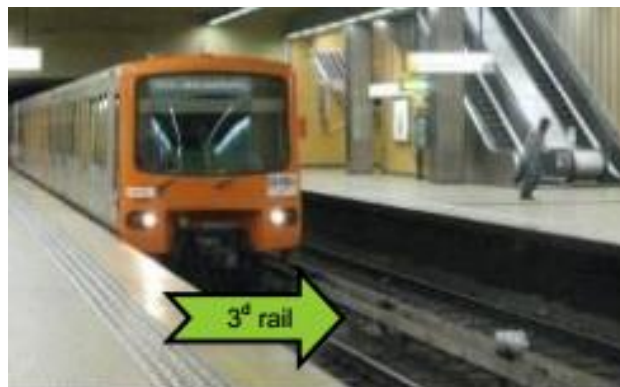
Figure 3.5: Third rail System
