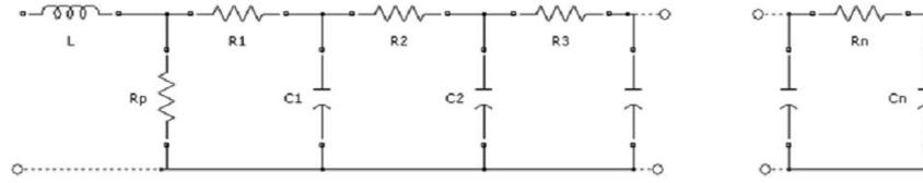
Figure 3.16: Equivalent circuit of a supercapacitor, realistic model
