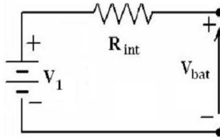
Figure 3.11: Schematic diagram of the  $R_{int}$  model.
