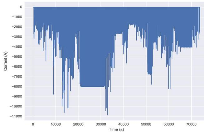
Figure 3.9: Metro line residual braking energy measurement
