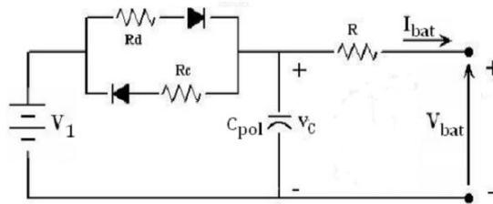
Figure 3.13: Dynamic Thevenin equivalent battery model scheme
