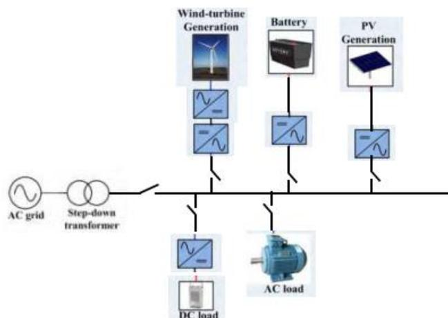
Figure 2.5: Radial, grid configurations
