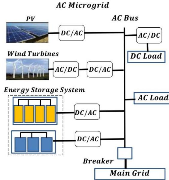
Figure 2.2: AC MicroGrid
