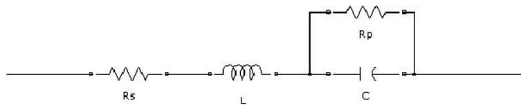
Figure 3.15: Equivalent circuit model of an supercapacitor
