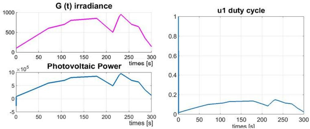
Figure 4.7: PV power with Varying Irradiance
