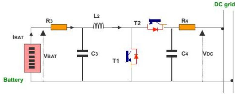
Figure 3.23: DC Bidirectional Converter Circuit
