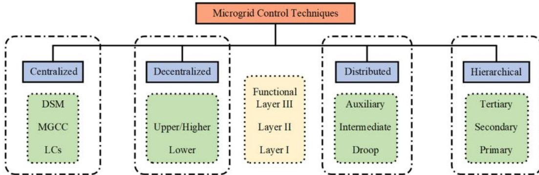
Figure 2.8: Classification of MicroGrid control techniques and functional layer structure
