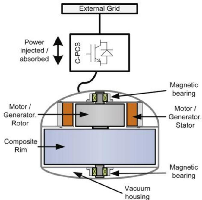
Figure 2.21: Topology of Flywheel Energy Storage System
