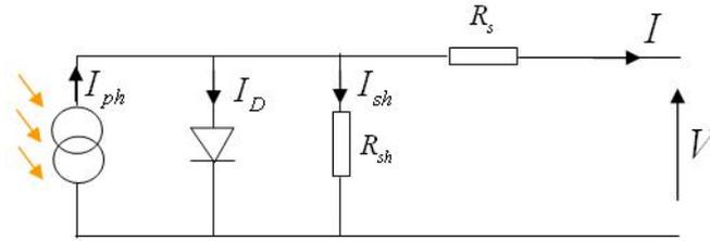
Figure 3.1: Equivalent circuit model of solar cell
