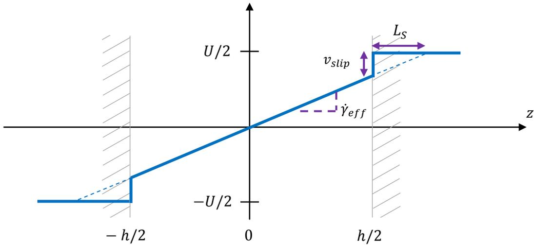
**Figure IV-7. Schematic definition of the slip length.
