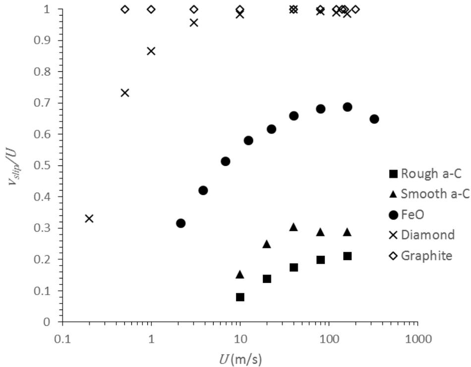
**Figure V-3. Ratio of the interfacial velocity slip on the imposed shearing velocity as a function of the imposed shearing velocity.**
