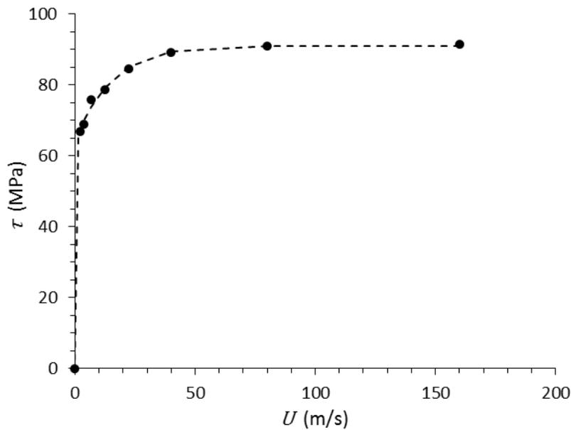
**Figure IV-4. Evolution of the global shear stress  $\tau$  in the lubricated contact as a function of the shear velocity, for an confining pressure of 500 MPa and a wall temperature of 350 K. The dashed line is a guide for the eyes.**
