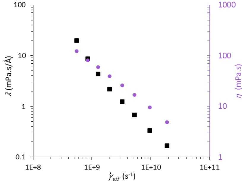
**Figure IV-9. Variation of the liquid/solid friction coefficient  $\lambda = \tau/v_{slip}$  at the IL/FeO interface in relation with the effective shear rate. By way of comparison, the viscosity is also reported on a secondary axis.**
