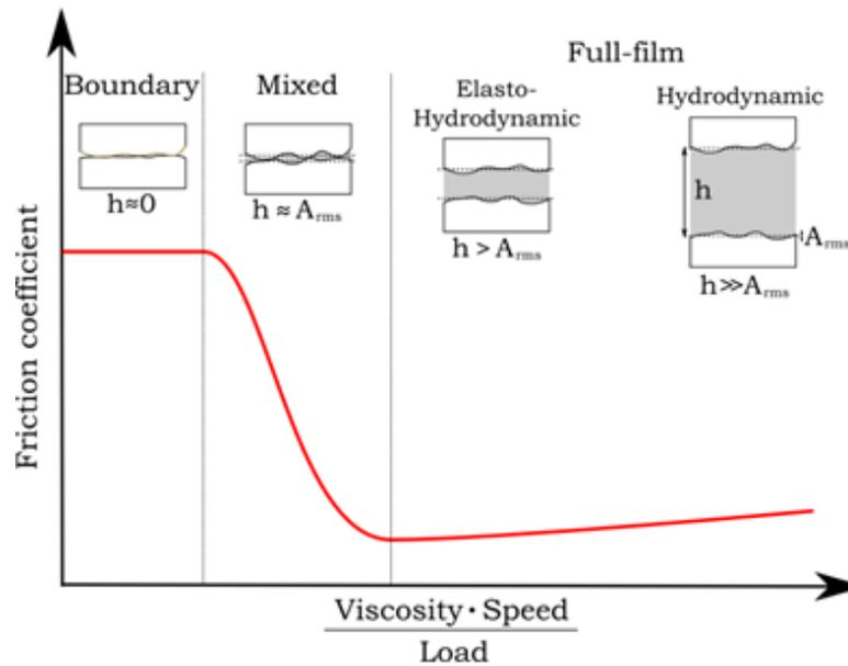
**Figure I-1: Stribeck curve, representing the qualitative dependence of the friction coefficient with operating conditions. A comparison between the contact thickness  $h$  and the root mean square roughness amplitude  $A_{rms}$  of the surfaces is also shown. From Savio [15].**
