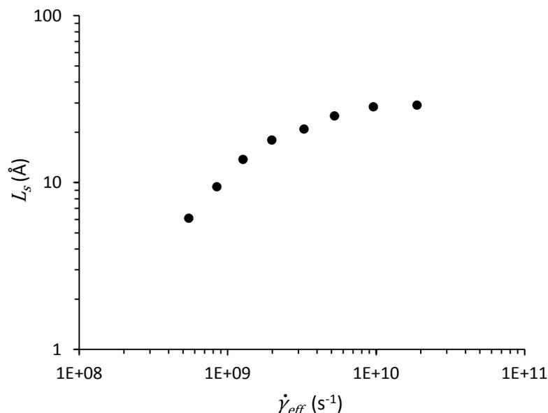
**Figure IV-8. Effective shear rate dependence of the slip length  $L_s = v_{slip}/\dot{\gamma}_{eff}$**
