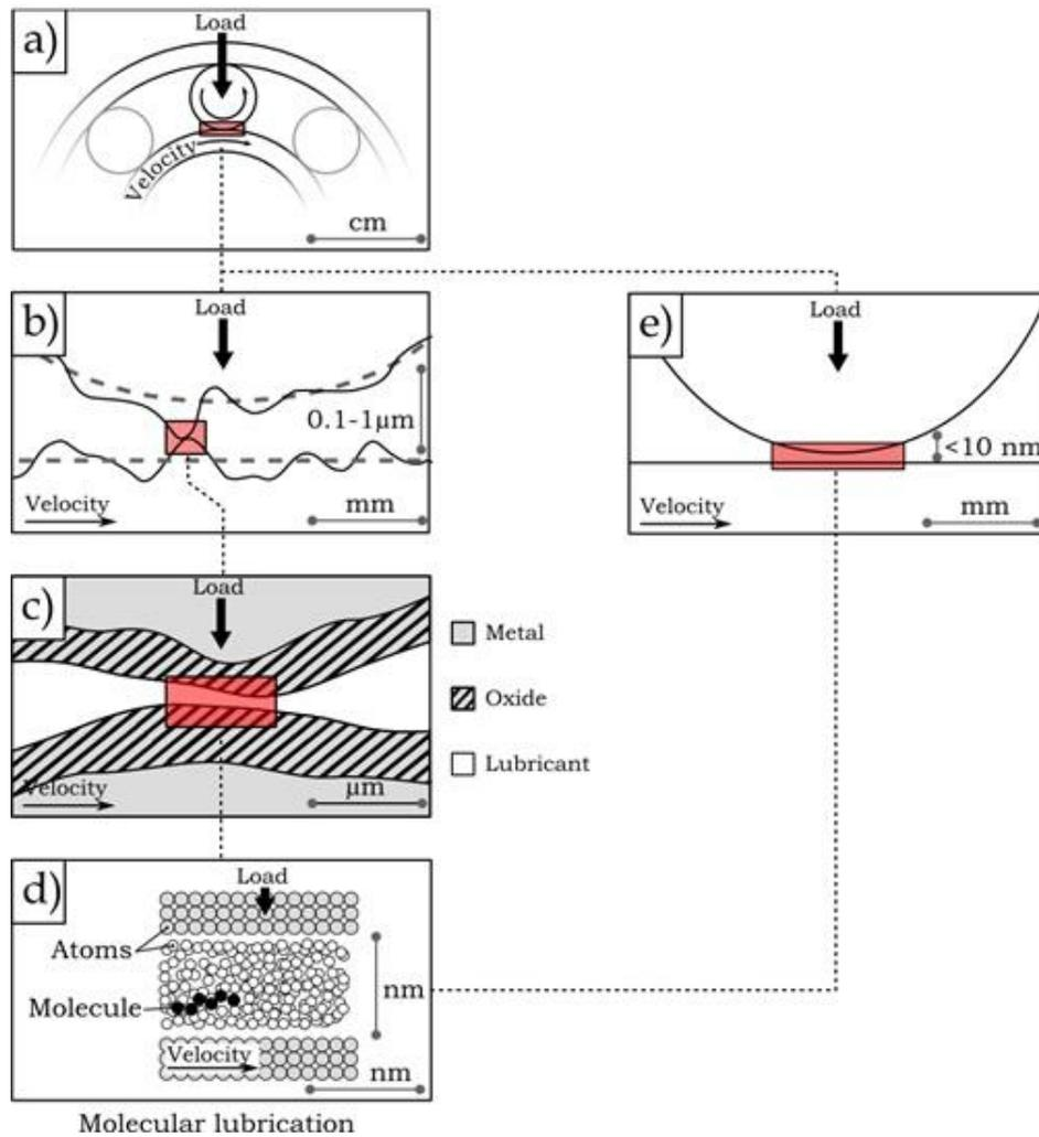
**Figure I-4: Multi-scale nature of a lubricated contact problem with film thickness reduction: from a macroscopic application to molecular lubrication between surface asperities (a → b → c → d) or between very smooth surfaces (a → e → d). From Savio [15].**
