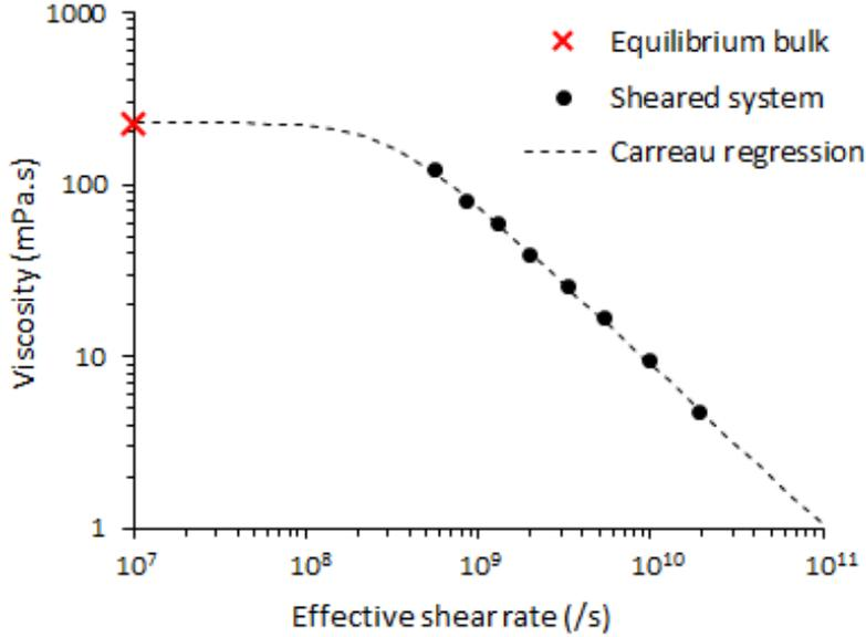
**Figure IV-6. Viscosity of the confined IL as a function of the effective shear rate  $\dot{\gamma}_{eff} = -dv/dz$  in the confined fluid. The dashed line is a Carreau regression of the viscosity. The red cross indicates the value of the Newtonian viscosity at 500 MPa and 350 K (Chapter III).**
