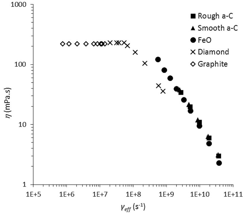
**Figure V-7. Viscosity with respect to the effective shear rate and the surface nature.**
