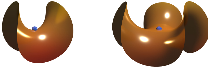
Figure 3.8 – Saddle points (blue spheres) of a 2-dimensional PL scalar field. A regular saddle (left) has an upper (resp. lower) link consisting of two connected components; whereas a multi-saddle may have more (right, three in this case).
