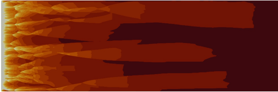
Figure 6.11 – Diffuse run example. The tips of fingers grow wider than their base, forming a sort of inverted funnels. The saturation field does not exhibit a very sharp frontier with the background.
