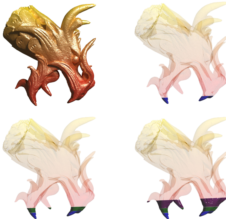
Figure 3.9 – Some nested complexes induced by the lower-star filtration of a PL scalar field (valuing from red to yellow) defined on a PL 3-manifold (the dragon’s head). Sub-complexes are shown in opacity at three filtration levels i (top right) < j (bottom left) < k (bottom right). A new connected component has appeared from \mathcal{L}(i) to \mathcal{L}(j) , just before it disappears at \mathcal{L}(k) . Another new connected component appears in \mathcal{L}(k) .
