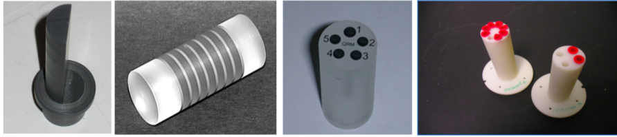
Figure 2.3: Phantoms used for the PIXSCAN characterization, from left to right: a spatial resolution phantom (based on the “edge method”), a phantom Deprise (QRM, Germany) for the evaluation of the reconstruction distortions, a linearity phantom (QRM, Germany) and two home made low contrast phantoms filled with iodine solutions at different concentrations.
