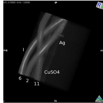
Fig. 14. 3D volume rendering of the slices acquired with Threshold 2 (25.5 keV) and reconstructed with FDK.
