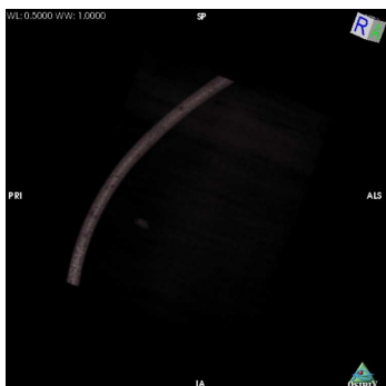
Fig. 16. 3D volume rendering of the subtracted windowed slices (E_{2I} - E_{3I}) - (E_{1I} - E_{2I}) magnifying the Iodine content of the twisted phantom.
