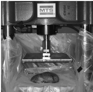
Fig B- 9. Experimental set up of uniaxial compression tests on human liver (Conte, 2012) On one hand, impact tests maintain a good geometry of the organ and a good restitution of the lesions (Sparks, 2007). On the other hand, it is possible to note an influence of the shape of the impactor and a difficult analysis of the stress-strain relationship.
