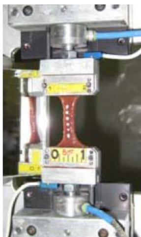
Fig B- 11. Experimental set up for tensile tests on bovine liver samples (Santiago, 2010)
