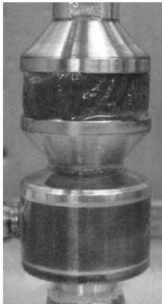
Fig B- 7. Uniaxial compression test on cylindrical porcine samples of 19 mm in diameter and 10 mm thick (Raghunathan, 2010)
