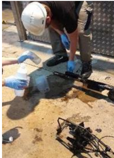
Figure 31. Visual inspection and cleaning of the quality sensors (photo: Duy Khiem Ly).
