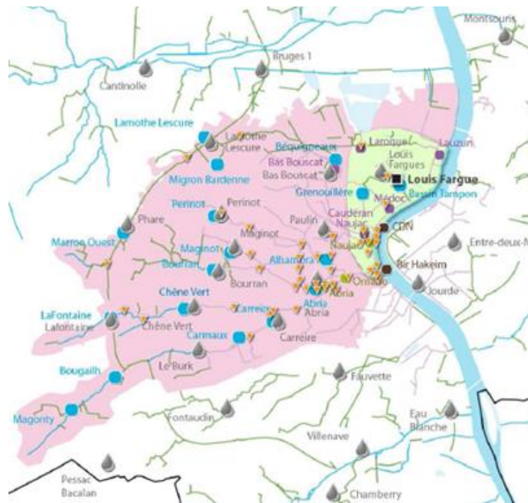
Figure 20. Louis Fargue catchment consists of the pink area (controlled by static or local dynamic rules) and the green area (under global control based on hydraulics) (after Maruéjols and Montserrat, 2016).
