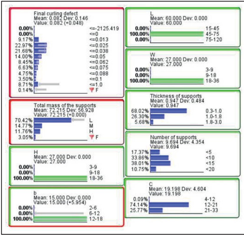
Figure 57. Predicted effect of part width and part height on the probability of curling defects for medium-sized parts (45 < L < 75) compared to Figure 56
