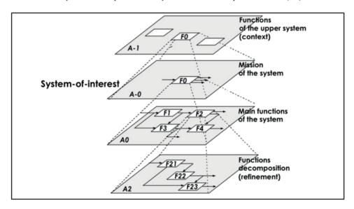
Figure 9. Function hierarchical decomposition (Faisandier, 2013)
