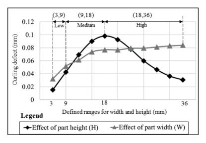
Figure 58. Effect of part height and part width on the curling defect
