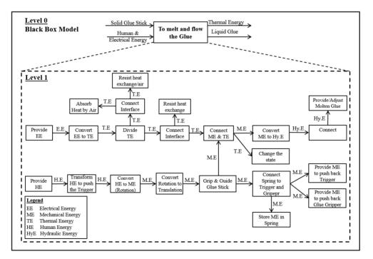
Figure 34. Functional model of glue gun using a reverse engineering approach (Publication III)
