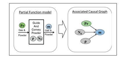
Figure 21. Left: An example of the functional model. Right: and its associated causal graph
