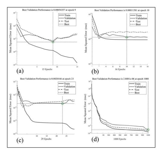
Figure 51. Performance curves for classical ANNs to model part's a) wall thickness, b) height, c) mass and d) performance curve for the best-fit scenario (standard function z=sin(x).cos(y)) (Nagarajan et al., 2019)
