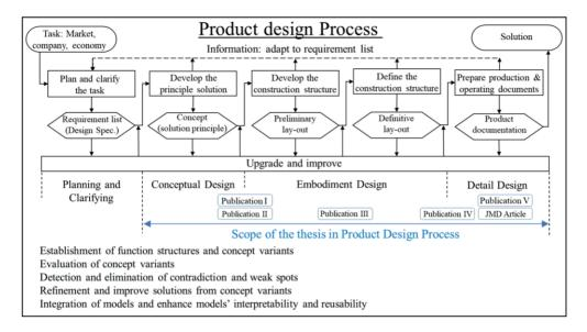
Figure 2. Product design process, re-arranged from (Pahl et al., 2007)
