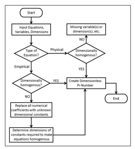
Figure 23. Description of the algorithm for equation integration
