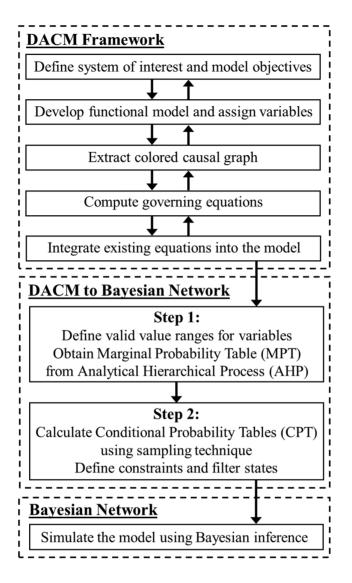
Figure 54. Proposed methodology workflow of the case study
