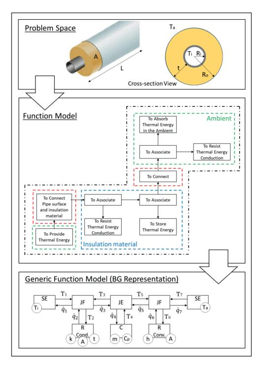
Figure 27. Function modeling for pipe insulation case study
