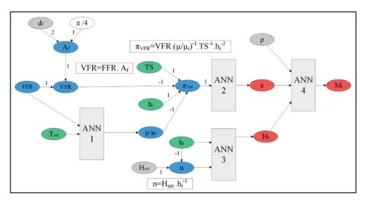
Figure 49. A simplified modular KB-ANN topology for the FDM process using causal graph developed by DACM framework (Nagarajan et al., 2019)
