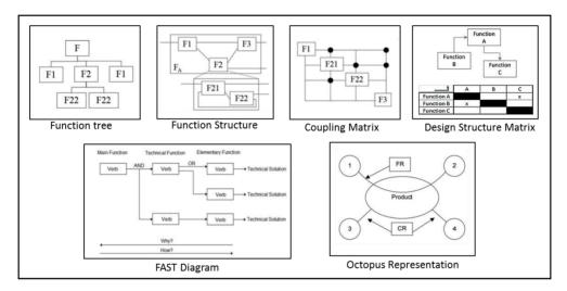
Figure 7. Different functional model representations
