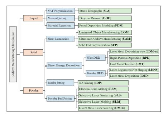
Figure 11. A classification for additive manufacturing processes
