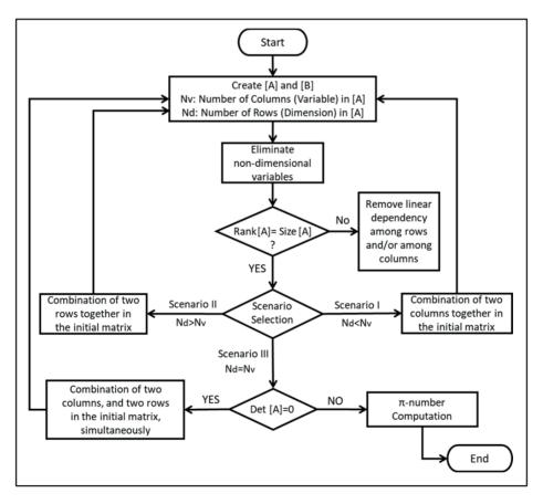
Figure 22. Description of the algorithm for non-singularity of [A]
