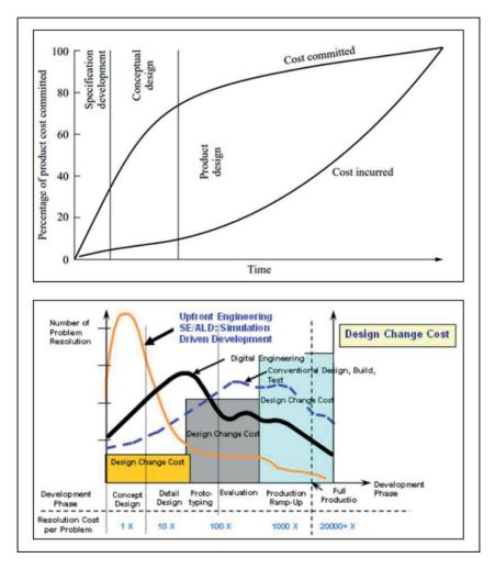
Figure 3. Top: Manufacturing costs during product design stages (Ullmann, 2015), Bottom: Cost of design change at different stages of PDP (Namouz, Summers, Mocko, & Obieglo, 2010) Furthermore, the cost of design changes in later phases is drastically increasing (Saravi, Newnes, Mileham, & Goh, 2008). Therefore, we are in the phase where activities are not costly but have a significant impact on the overall cost and product's success.
