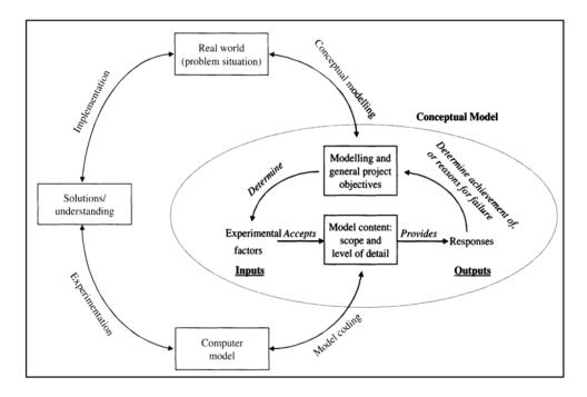
Figure 4. Conceptual modeling in simulation process (Robinson, 2004)
