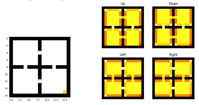
Figure 6.2: Left: Four-room grid-world (left) with walls in black, and goal state in yellow. Right: equivalence classes for state-action pairs (one color per class).
