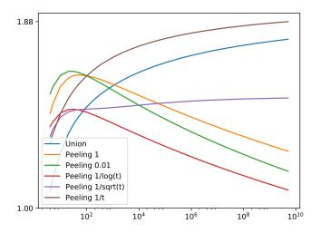
Figure 2.1: Ratio of different time-uniform concentration bounds over that of the Laplace method, as a function of t, for a confidence level  $\delta=0.01$  and various choice of  $\eta=\eta(t)$ . This indicates that all other bounds are larger than the Laplace bound by a multiplicative factor up to 1.88 here, and none is smaller until at least time  $t=10^{10}$ . Notice the logarithmic scale.
