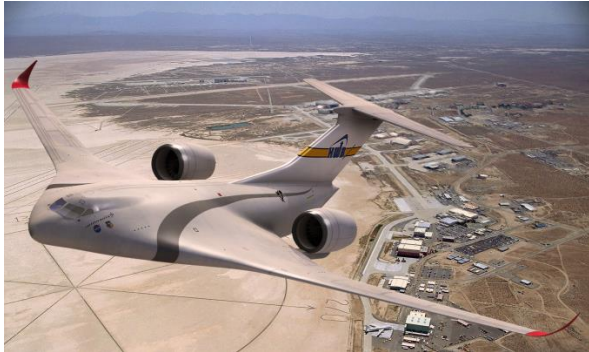
Figure 18: Hybrid Wing Body configuration proposed by Lockheed Martin [83]
