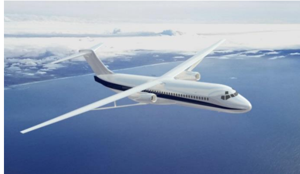
Figure 19: Transonic Truss-Braced Wing suggested by Boeing [83]
