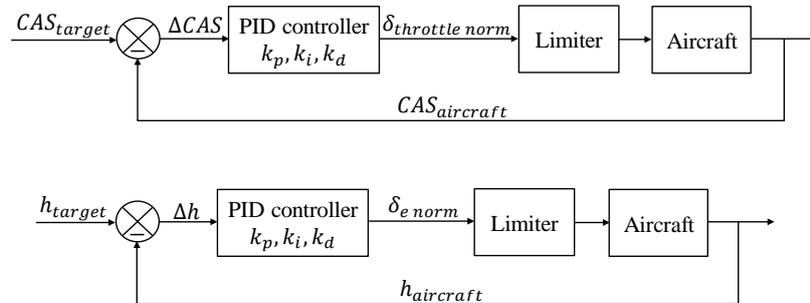
Figure 99: Speed hold (top) and altitude hold (bottom) control systems for cruise phase
