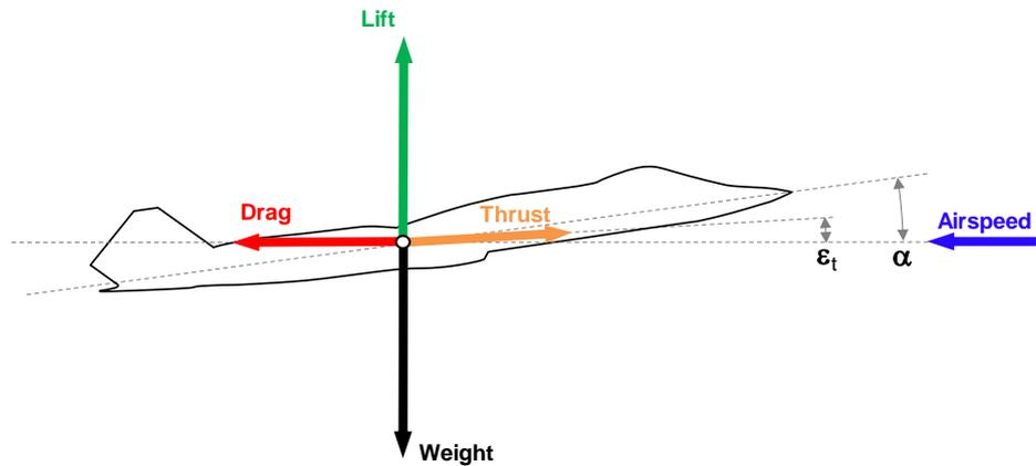
Figure 10: Forces applied during steady flight
