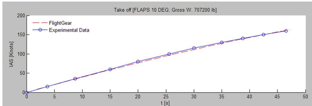
Figure 87: Comparison of Boeing B747-100 experimental data and FlightGear simulations [229]
