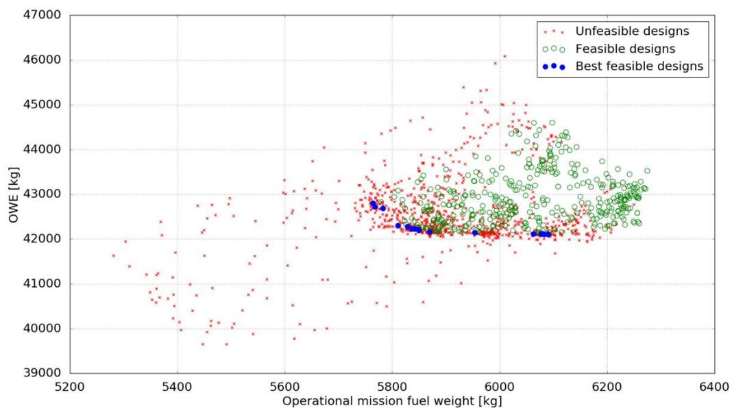
Figure 81: Exploration of the design space during the FAST MDAO process - Optimization 4
