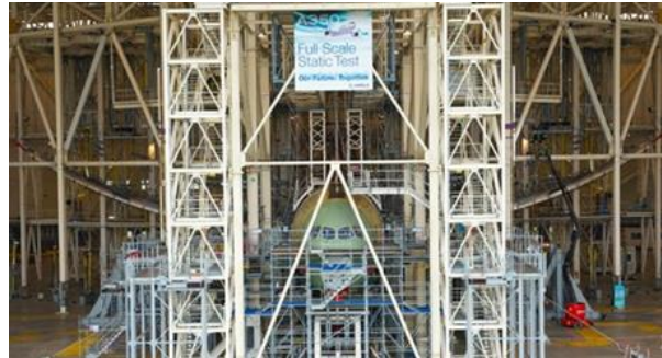
Figure 6: Airbus A350 full scale wing static test [42]
