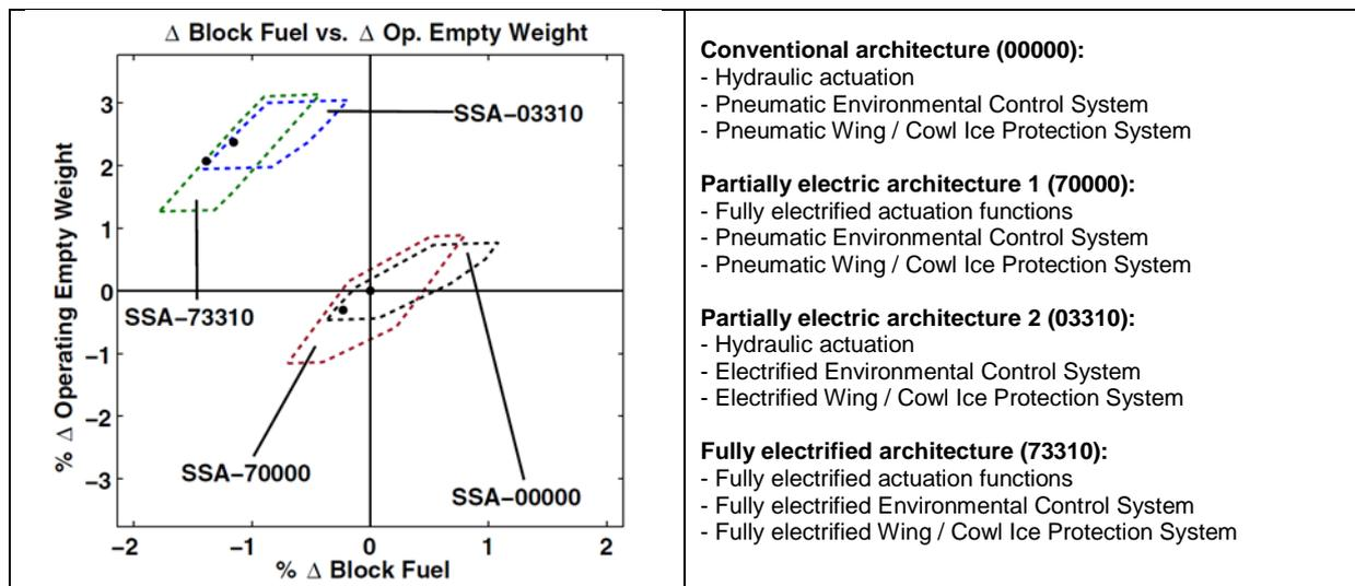
Figure 29: Sensitivity of different aircraft subsystem architectures [143]
