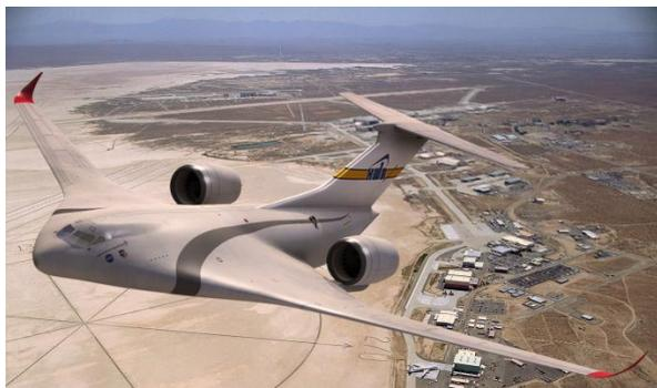
Figure 18: Hybrid Wing Body configuration proposed by Lockheed Martin [83]
