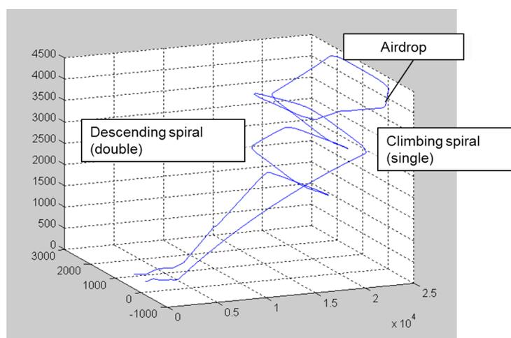
Figure 45: Reference mission for the EOLE demonstrator [175]
