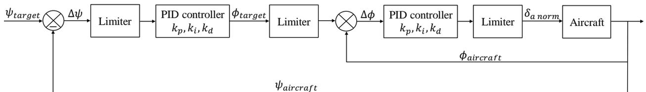
Figure 100: Heading hold control system (for all segments)
