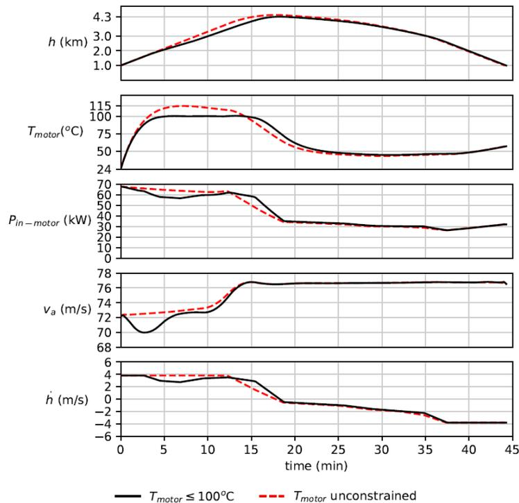
Figure 28: Optimized flight profiles with and without constraints on motor temperature [139]
