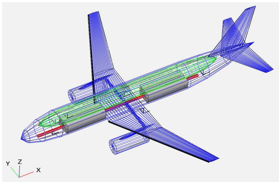
Figure 95: OpenVSP model including the new volumes representing mass distribution ( $V_1$  is highlighted in red,  $V_2$  and  $V_3$  are colored in blue,  $V_4$  and  $V_5$  are represented in black,  $V_6$  and  $V_7$  are the grey blocks while  $V_8$  is shown in green)
