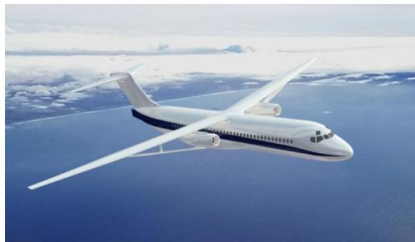
Figure 19: Transonic Truss-Braced Wing suggested by Boeing [83]
