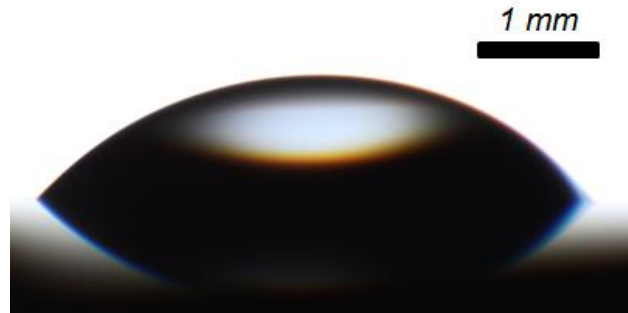
Figure 2.4. Image of the contact between the water droplet and the sample of Ge.
