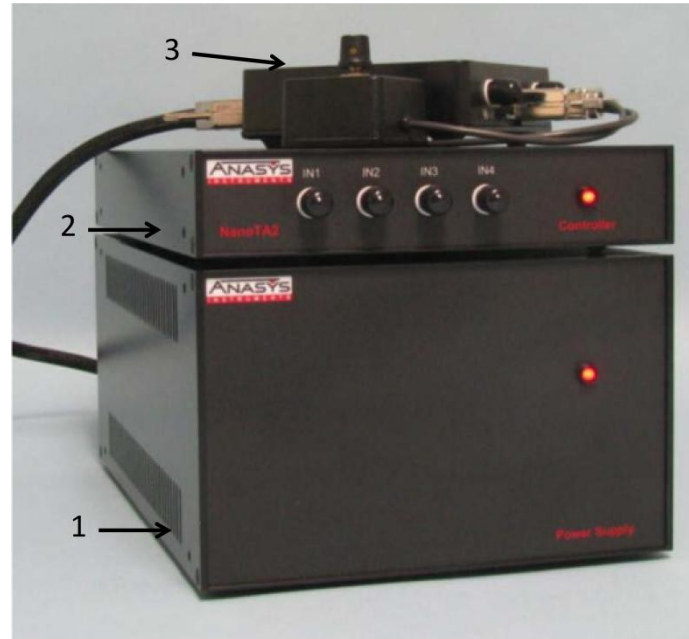
Figure A.6. The three parts of the NanoTA2: 1) Power supply, 2) Controller and 3) CAL Box.
