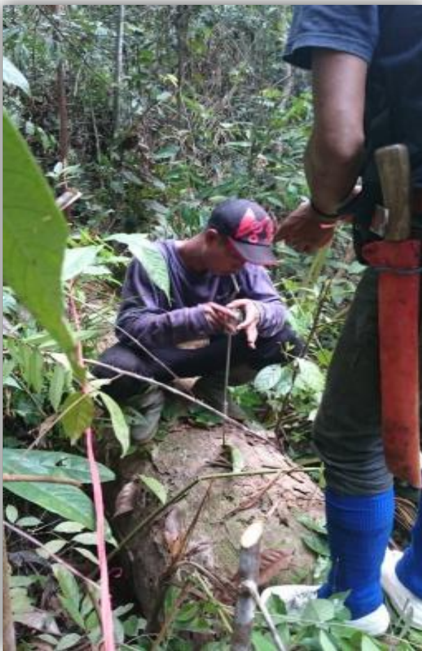
Measuring specific density of fallen deadwood using a dynamic penetrometer in a Dipterocarp forest (Berau, East Kalimantan)
