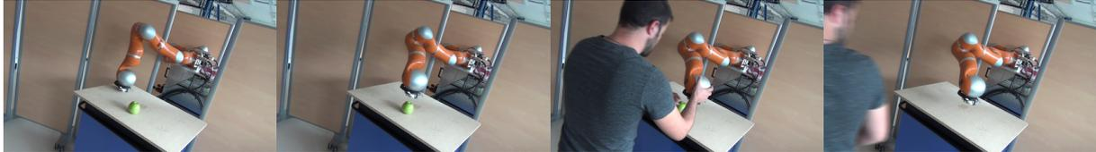
(e) Force control is performed at the first waypoint. (f) The robot avoids the obstacle by using repulsive potential fields. (g) The operator stops the robot to access the workspace. (h) The robot returns to the initial pose.
