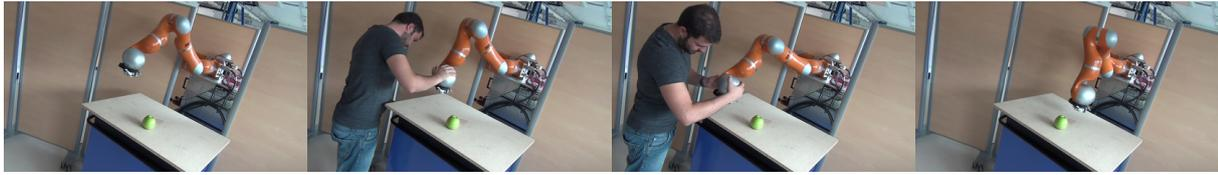
(a) The robot is waiting in its initial position. (b) The operator teaches the first waypoint. (c) The operator teaches the second waypoint. (d) The robots goes to the first waypoint.
