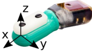
Figure 4.8 – BioTac with its attached reference frame.
