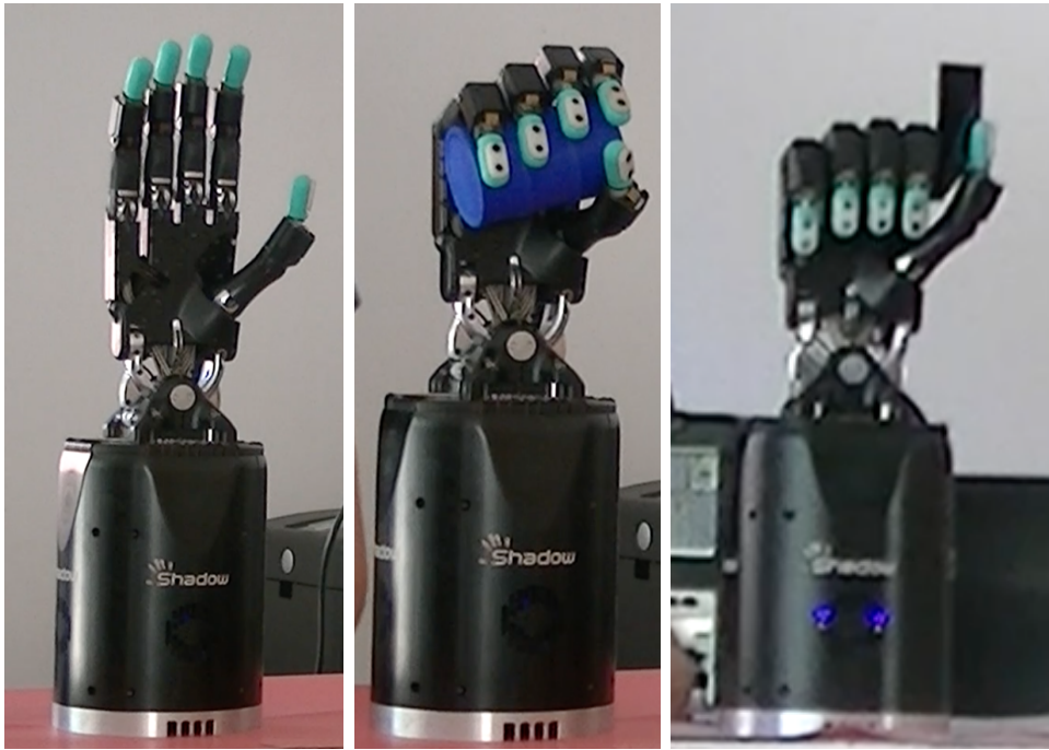
Figure 4.14 – Hand configurations. From left to right: open hand, palmar pinch and key-grip.
