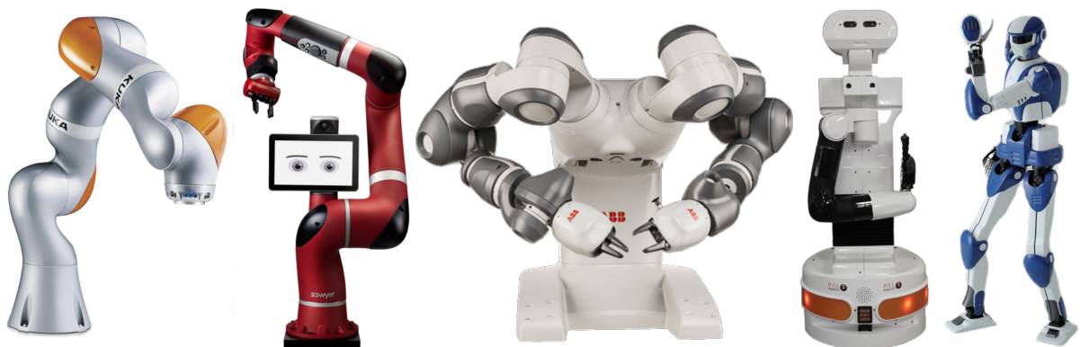
Figure 1 – Examples of lightweight robots, from left to right: Kuka LBR iiwa (2013), Rethink Robotics Sawyer (2015), ABB YuMi (2015), Pal Robotics TIAGo (2015), Kawada Industries HRP-4 (2011).
