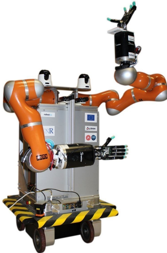
Figure 4.5 – The Bazar mobile manipulator.
