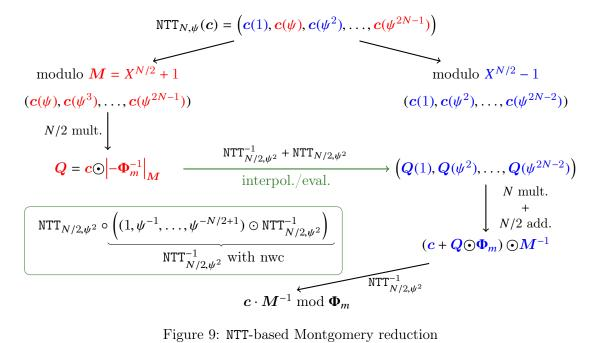
Figure 9: NTT-based Montgomery reduction
