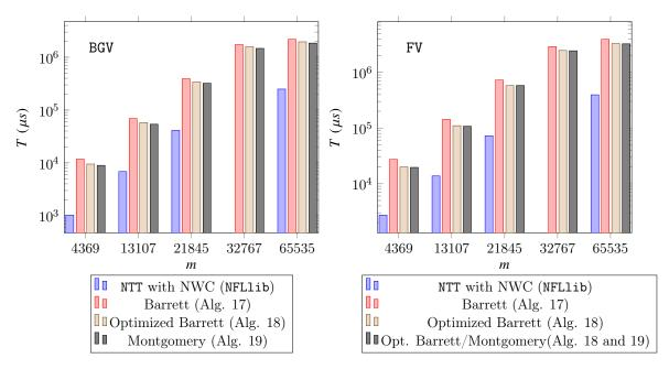
Figure 11: Execution time  $T(\mu s)$  for the multiplication plus relinearization of BGV and FV with several reduction strategies (plus modulus switching for BGV) on the m-th cyclotomic polynomial. Modulus q is a product of 62-bit prime moduli and y-axis is in logarithmic scale.
