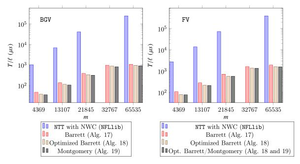
Figure 12: Execution time per slot  $T/\ell$  ( $\mu s$ ) for the multiplication plus relinearization of BGV and FV with several reduction strategies (plus modulus switching for BGV) on the m-th cyclotomic polynomial. Modulus q is a product of 62-bit prime moduli and the y-axis is in logarithmic scale
