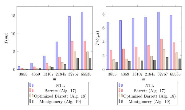
Figure 10: Execution time T(ms) (resp. per batching slot  $T/\ell$  ( $\mu s$ )) for multiple reduction strategies for cyclotomic polynomials of index m on a single 62-bit modulus.
