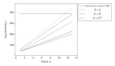
Figure 5: Example of noise growth, for  $n = 2^{13}$ ,  $\log_2(q) = 390$  ( $\nu = 30, k = 13$ ),  $t = 2, \sigma_{err} = 8$ ,  $B_{key} = 1$  (dashed line: theoretical bound, using (2.4.1); plain line: measurements).
