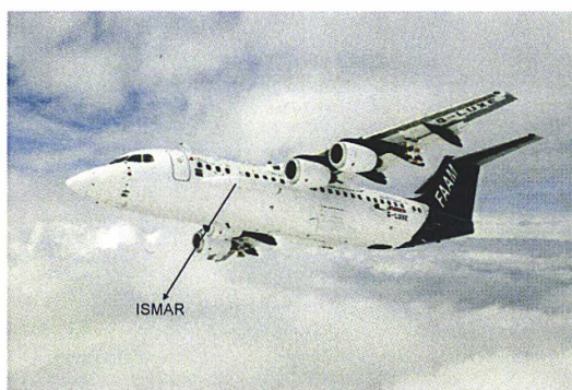
Figure 7.1: The BAe FAAM aircraft showing the position of ISMAR.
