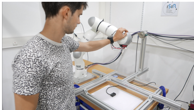
FIGURE 4.6: Physical interaction with the robot. An operator restrains the robot motion along its y-axis.
