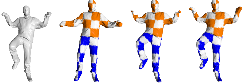
Figure 4.6 – Our E_c energy term prevents loss of tracking. From left to right: \mathcal{S} , \mathcal{T} , template deformation without E_c , and with E_c .
