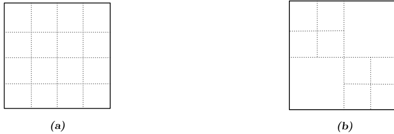
Figure 4.4: (a) Block cluster representation \mathcal{T}_{I \times I} for the illustrative example (full structure); (b) Hierarchical partition \mathcal{P} \subset \mathcal{T}_{I \times I} of the same matrix based on the admissibility condition (sparse structure).
