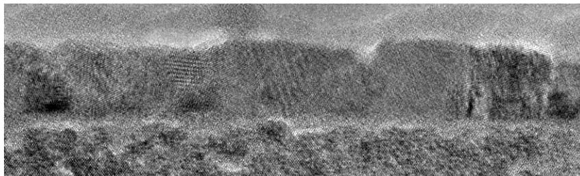
13 nm La-ZrO<sub>2</sub> recuit 400°C 60s sous N<sub>2</sub>
