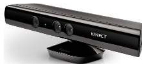
(e) Camera RGB-D (Kinect – Microsoft)
