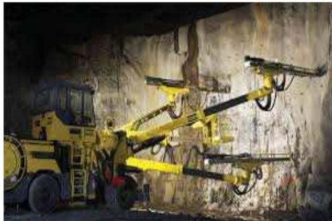
FIGURE 1.15 – Machine jumbo
