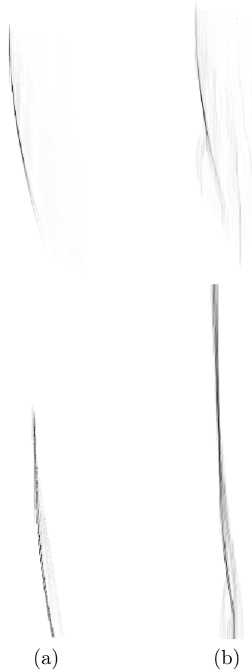
FIGURE 3.27: Comparison between original voting spaces created from ground truth of optical flow (a) and estimated optical flow (b). Top line shows c -velocity voting space for horizontal plane. Bottom line displays the \mathbf{V} voting space
