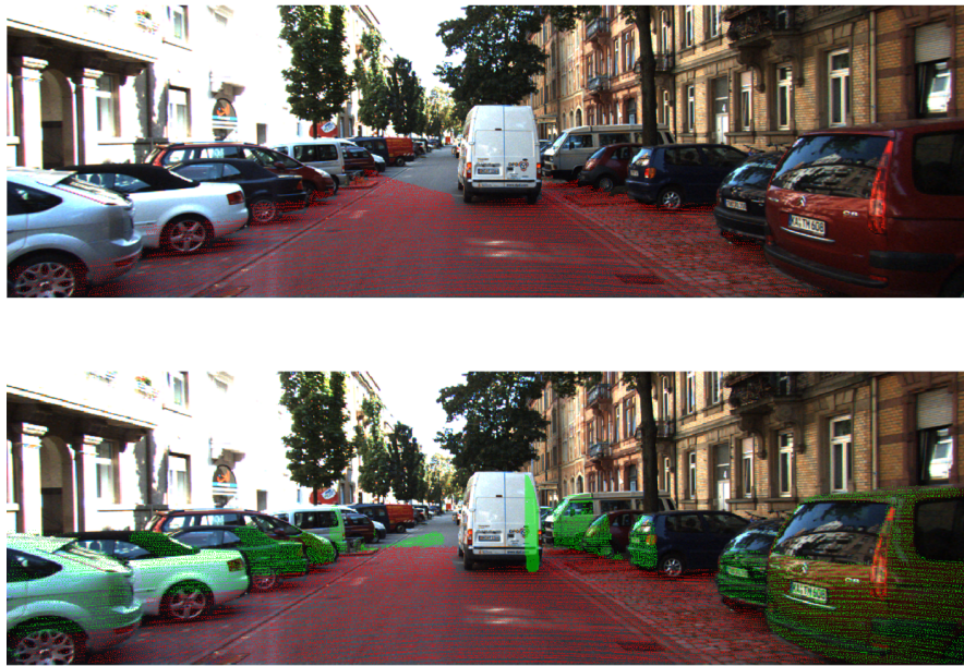
FIGURE 3.26: Segmented image according to the found parabola for c -velocity (top) and uv -velocity (bottom) on the ground truth OF. The horizontal plane is drawn in red
