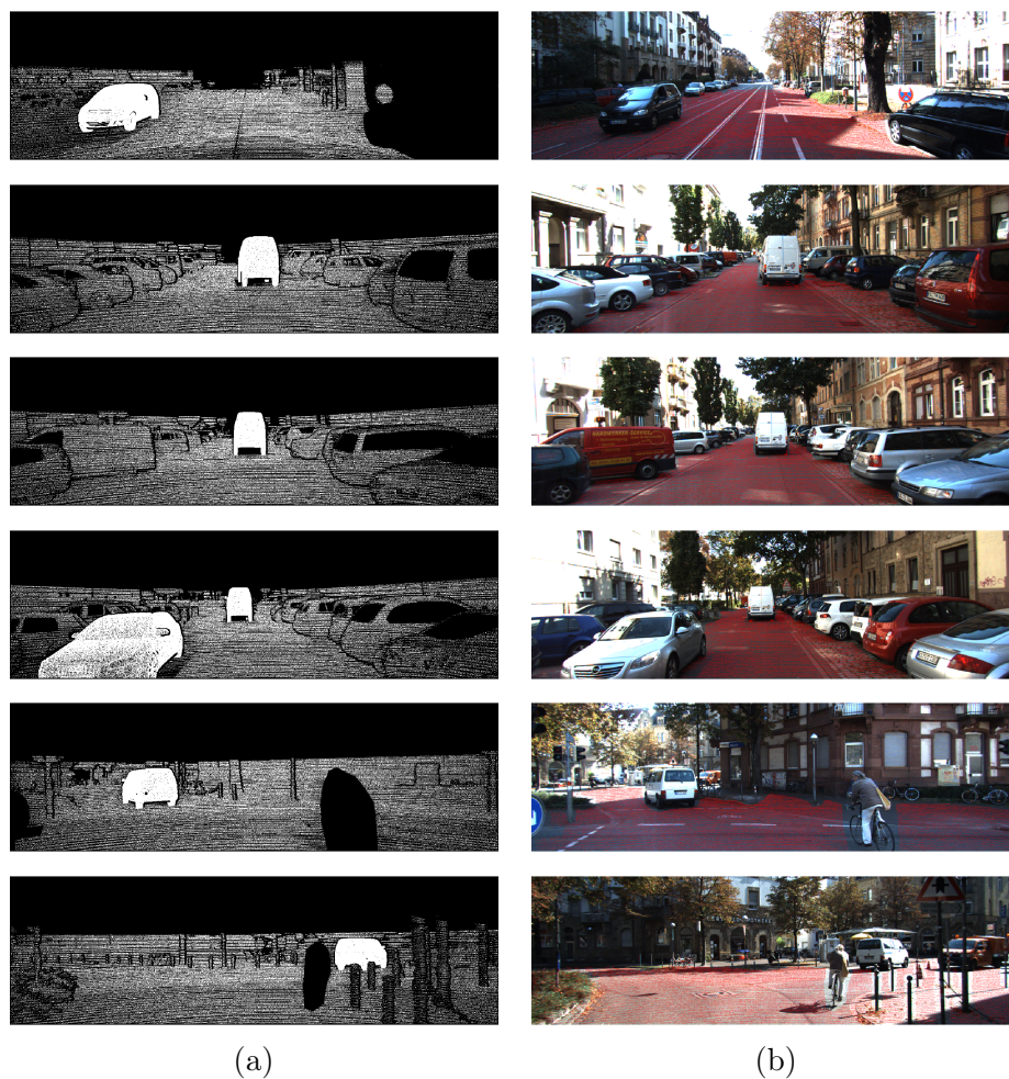
FIGURE 3.33: The mask of available ground truth optical flow (a) and the ground truth of segmentation for horizontal plane (b) for 6 sequences indexed (1),(2),(3),(4),(5),(6) respectively from top to bottom
