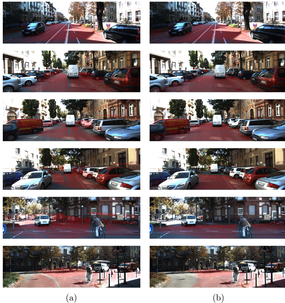
FIGURE 3.34: The segmentation results from a parametric method (a) and our voting method (b).
