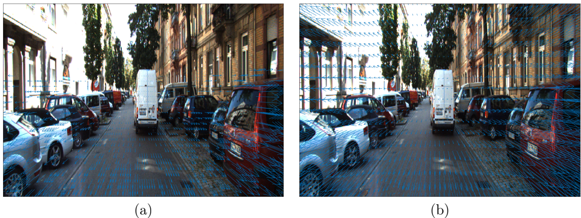
FIGURE 3.21: The ground truth (a) and the estimated OF (b) of the sequence.
