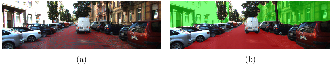
FIGURE 3.22: The ground truth of segmentation (red for horizontal plane, green for lateral plane) for sparse ground truth optical flow (a) and dense optical flow (b).
