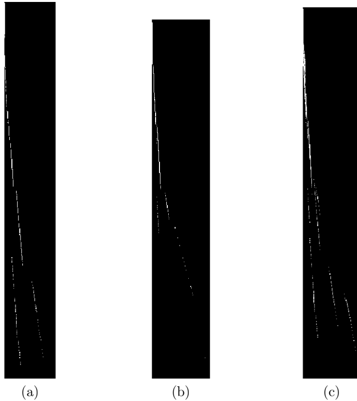
FIGURE 3.24: The lateral voting space for half-left (a) and half-right (b) and frontal voting space (c) for OF in figure 3.21(a). No parabola is found on these voting spaces. The horizontal axis represents the w -value and the vertical axis represents the c -values
