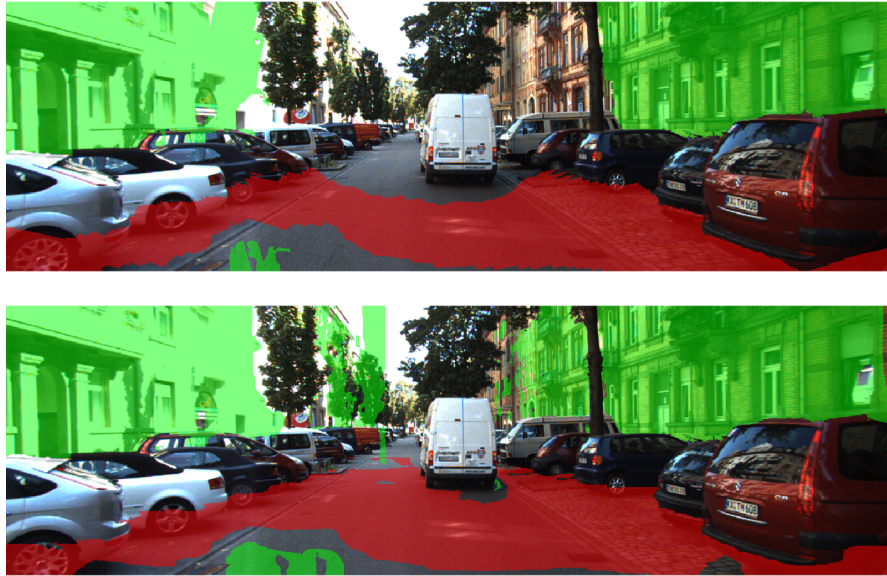
FIGURE 3.31: Segmented image according to the detected parabola for c -velocity (top) and uv -velocity (bottom) on the estimated OF . The horizontal plane is drawn in red, the lateral plane is coloured in green.
