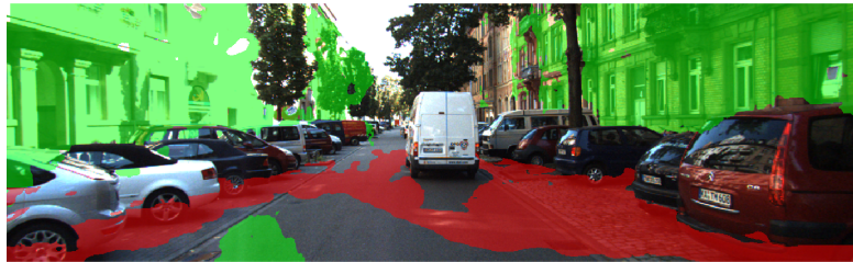
FIGURE 4.2: Example of segmentation result coming from the analysis of the uv -velocity computed from the proposed optical flow estimation.
