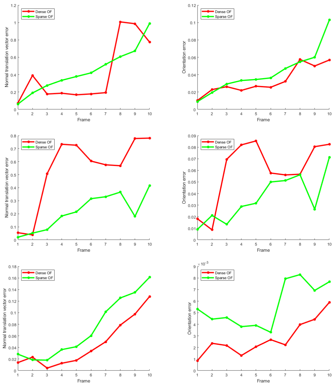
FIGURE 5.5: Evolution of the two measures : (a) translation direction and (b) orientation of camera on 3 sequences I,II,III from top to bottom respectively
