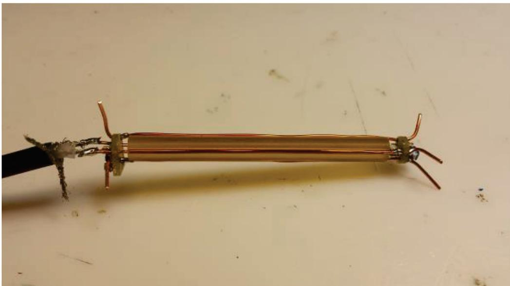
FIGURE V-17 : PROTOTYPE DE CAPTEUR ENDOLUMINAL A DOUBLE RESONANCE PROTON ET PHOSPHORE
