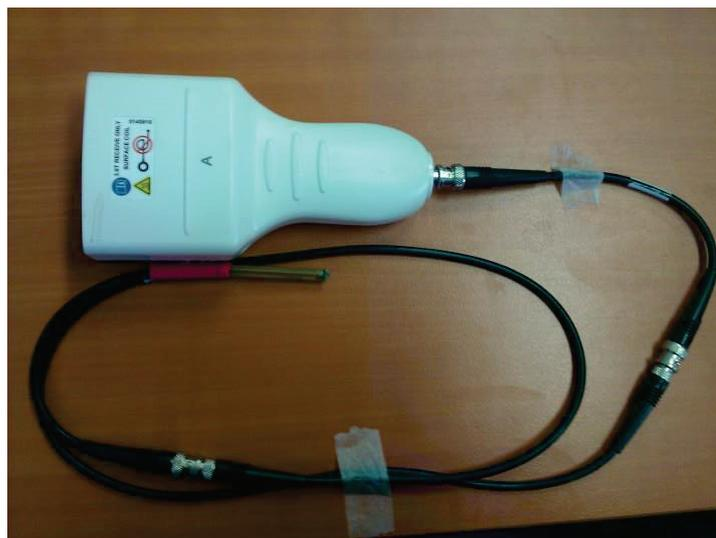
FIGURE VII-4 : CONNECTEUR GPFLEX INITIAL DISPOSANT D'UN UNIQUE CANAL DE RÉCEPTION PERMETTANT LA CONNEXION D'UN CAPTEUR ENDOLUMINAL DE RÉCEPTION
