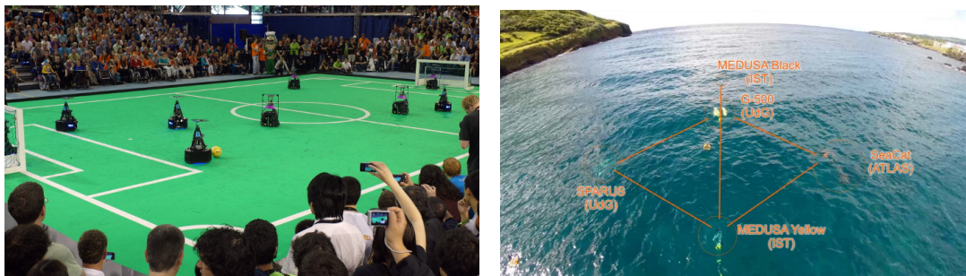
(a) Mobile robot teams competing in soccer. (b) Cooperative Formation Control in the EC MORPH Project (Abreu et al. , 2015)
