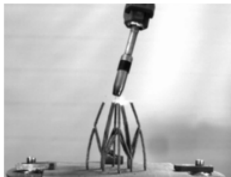
FIGURE 5.22 – Procédé de fabrication additive appelé Wire Arc Additive Manufacturing
