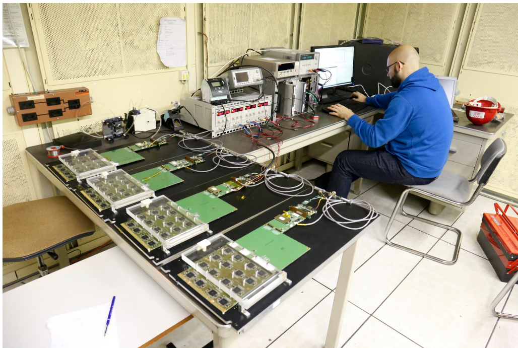
Figure 5.3 – Four FEV11 technological prototype slabs during November'15 tests at CERN.
