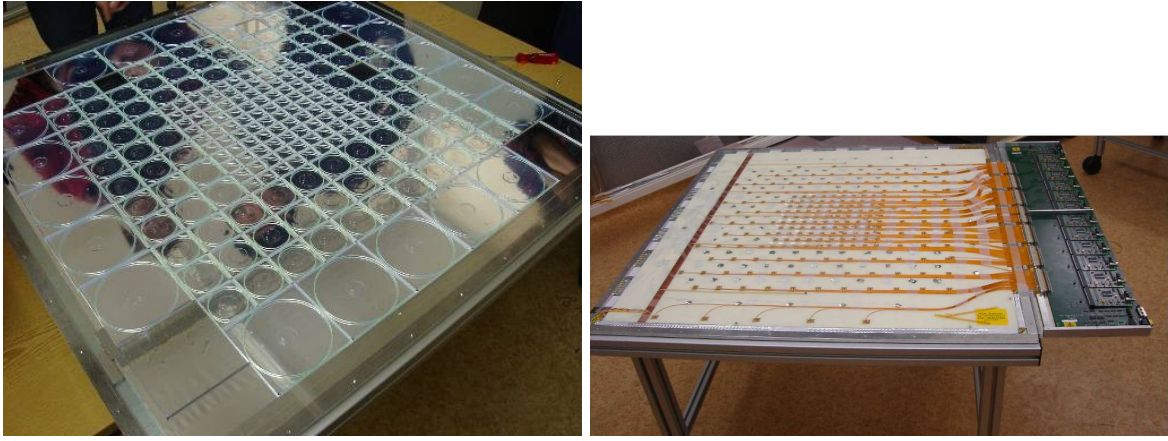
Figure 3.13 – One scintillator layer of AHCAL physics prototype before assembly (left) and the readout electronics (right).
