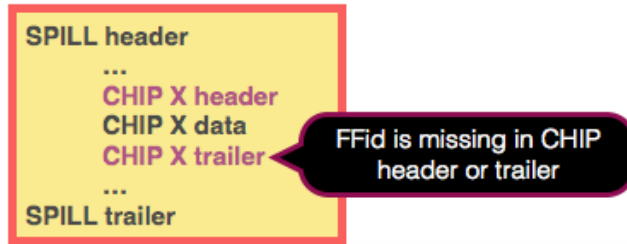
Figure 5.44 – FF CHIPid number can be missing in header or/and trailer of the CHIP DATA block.
