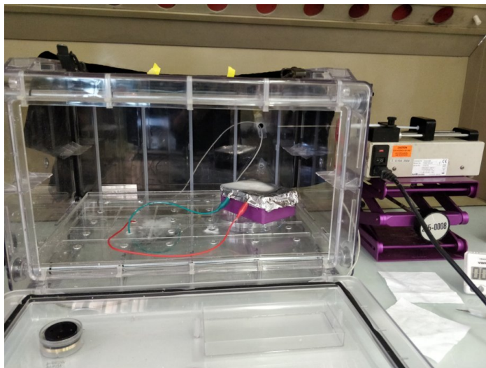
Figure 6.3: Vertical Electrospinning Setup
