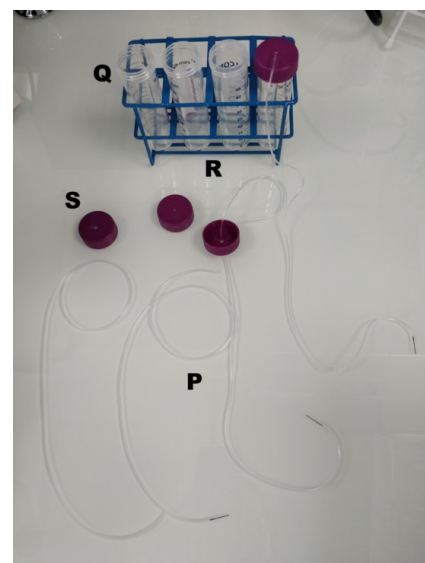
Figure 6.9: Preparing the reservoirs for medium collection
