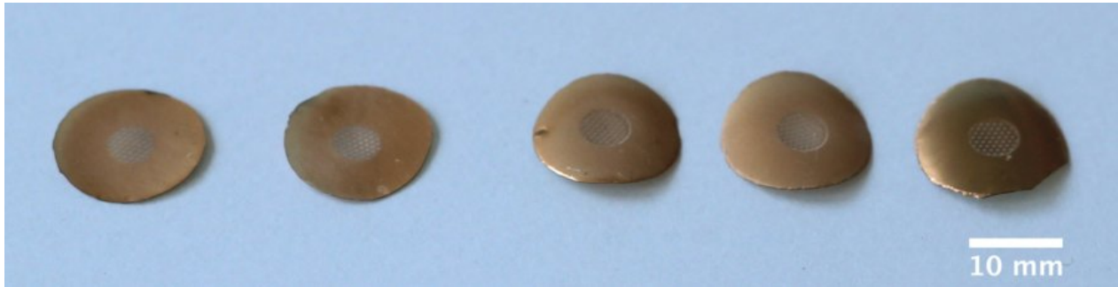
Figure 2.13: Depending on the fabrication process, the patches can be more (right) or less (left) flat. This was an important focus in our optimization of the fabrication process.
