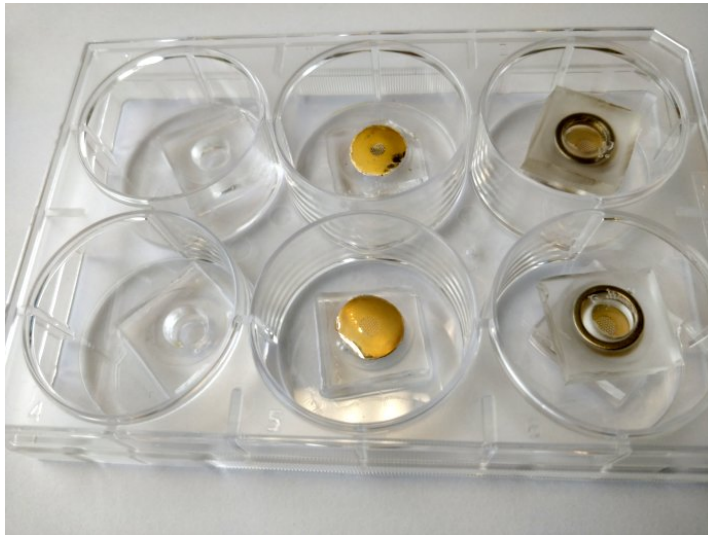
(a) Mounting PDMS-magnetic chamber: first three steps
