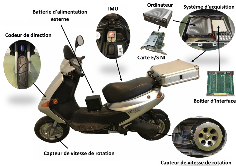
FIGURE 1.16 – Instrumentation du Scooter Peugeot
