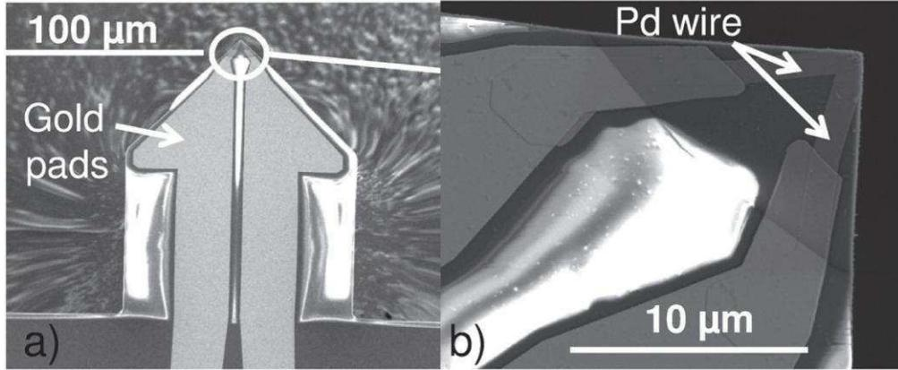
**Figure 2.** SEM images of the used KNT probe: (a) probe cantilever and (b) probe apex, where a V-shaped Pd wire is deposited on a  $\text{Si}_3\text{N}_4$  cantilever.
