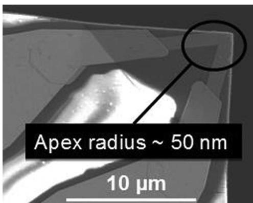
**Figure 4** SEM image of a palladium probe.
