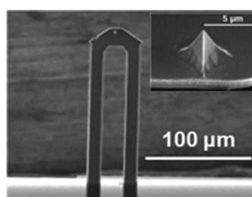
**Figure 5** SEM image of a doped silicon probe.
