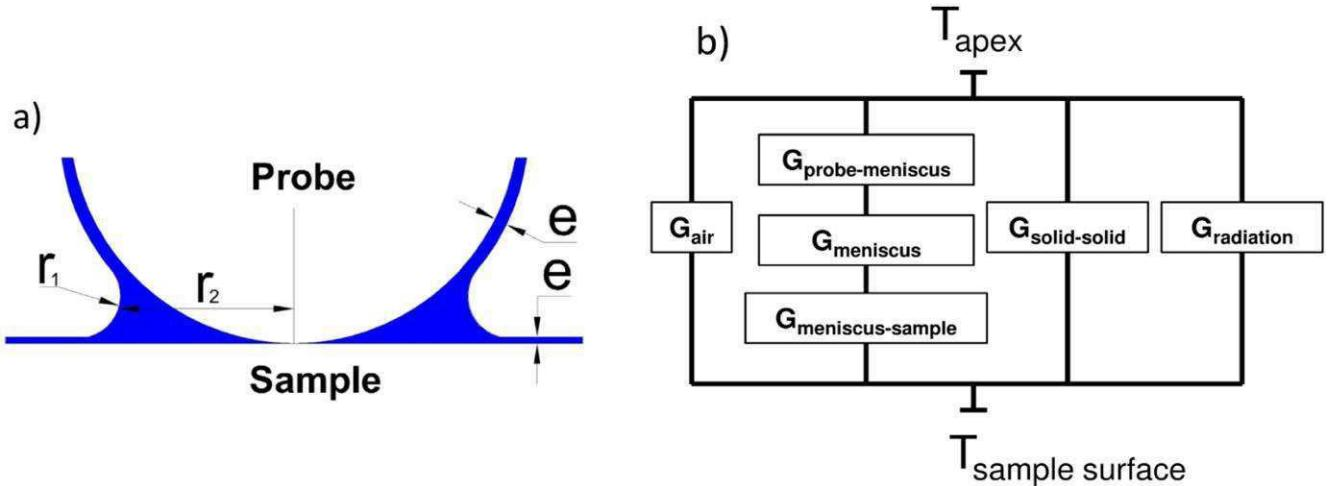
**Figure 1.** (a) Schematic of the water meniscus at the tip–sample contact and (b) description of the series of the thermal conductances between the tip apex and the sample surface.  $G_{\text{air}}$ ,  $G_{\text{solid-solid}}$ , and  $G_{\text{radiation}}$  are, respectively, the thermal conductances of air, solid–solid contact, and radiation.
