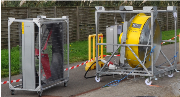
Fig. 3.2 – View of the two fans, TROTEC TTW 45000 : 2 m/s (left) and TROTEC TTW 100000 : 5 m/s and 8 m/s (right)
