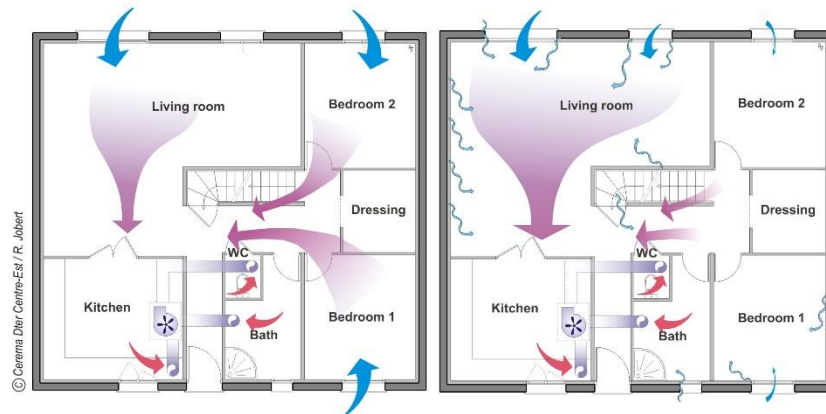
Figure 1. (a) Theoretical ventilation airflows in a dwelling and (b) short-circuiting due to non-uniformly distributed envelope airleakage. Source: (Carrié et al. 2006).
