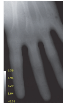
(b) Proton CT image of an hand phantom. In Plautz et al. 2014.
