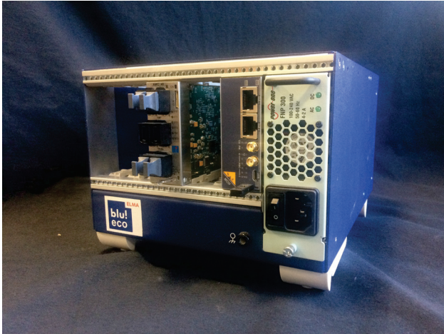
(a) \mu -TCA crate with the AMC40 board.
