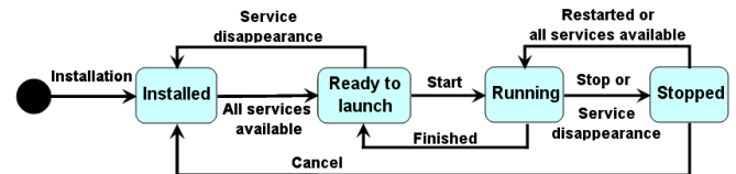
Figure 6. State diagram of scenario life-cycle
