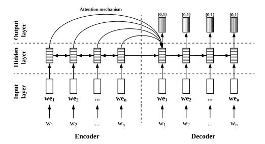
**Figure 5.2:** The words are represented by the word embedding representations in the input layer. The attention mechanism improves the decode processing. The output layer is composed of 0 (remove), 1 (remain) or <pad>.
