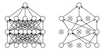
*Figure 2.13:* A dropout example (Source: (Srivastava et al., 2014)).
