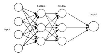
*Figure 2.7:* An example of a deep FeedForward Neural Network with 2 hidden layers.
