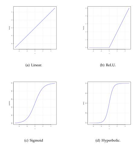
Figure 2.11: Plot of activation functions.
