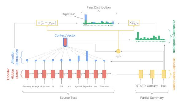
*Figure 2.15:* Pointer-generator model. The probability  $p_{gen} \in [0,1]$  is calculated at each decoder time step to generate a word from the vocabulary or copying a word from the source text (Source: (See et al., 2017)).
