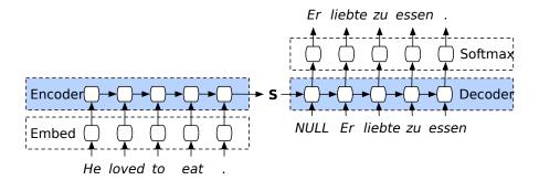
Figure 2.18: Neural machine translation example using a sequence-to-sequence model (Source: https://smerity.com/articles/2016/google\_nmt\_arch.html).
