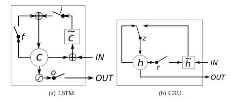
**Figure 2.10:** Illustration of (a) LSTM and (b) GRU. (a) i, f and o are the input, forget and output gates, respectively. c and  $\tilde{c}$  denote the memory cell and the new memory cell content. (b) r and z are the reset and update gates, and h and  $\tilde{h}$  are the activation and the candidate activation (Source: (Chung et al., 2014)).
