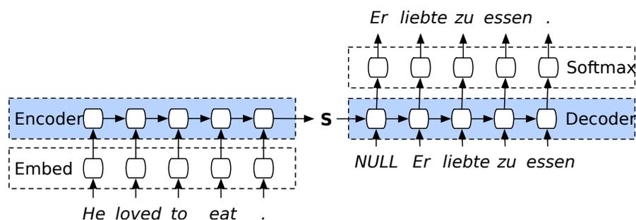
**Figure 2.18:** Neural machine translation example using a sequence-to-sequence model (Source: [https://smerity.com/articles/2016/google\\_nmt\\_arch.html](https://smerity.com/articles/2016/google_nmt_arch.html)).
