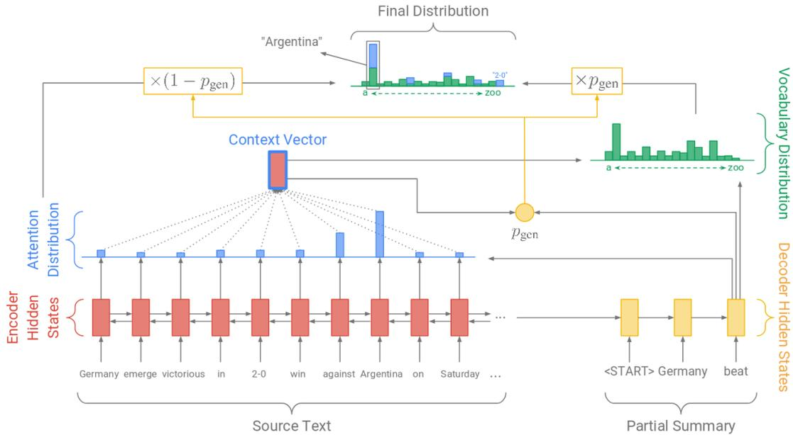
**Figure 2.15:** Pointer-generator model. The probability  $p_{gen} \in [0, 1]$  is calculated at each decoder time step to generate a word from the vocabulary or copying a word from the source text (Source: (See et al., 2017)).
