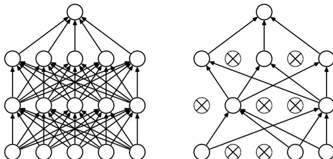
Figure 2.13: A dropout example (Source: (Srivastava et al., 2014)).
