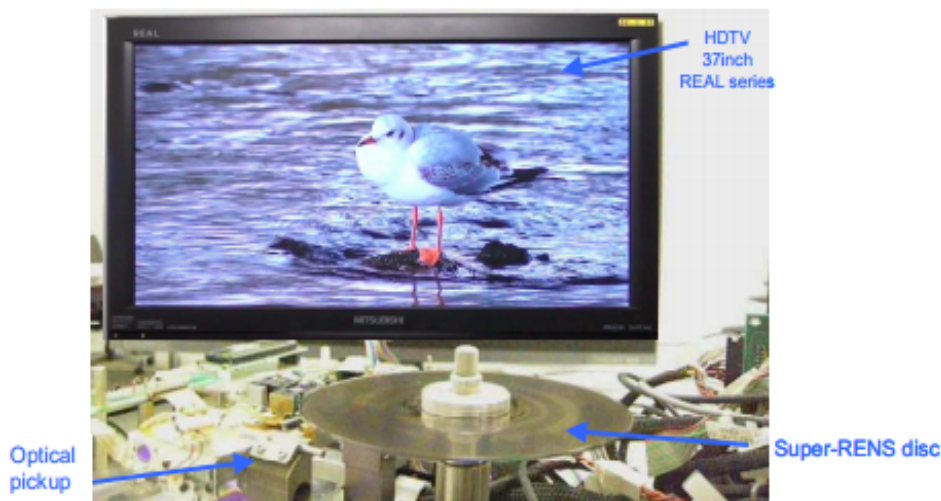
Figure 18: Demonstration of a Super-RENS single-face Blu-ray disc of 50Gb capacity in 2009.
