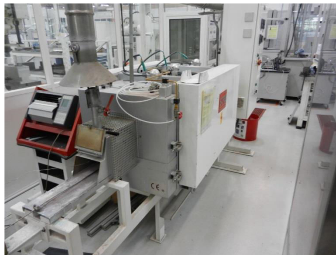
Figure 2.18. Prototype of the furnace used for the brazing process at Valeo.
