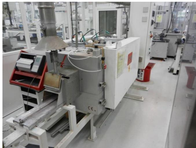
Figure 2.18. Prototype of the furnace used for the brazing process at Valeo.
