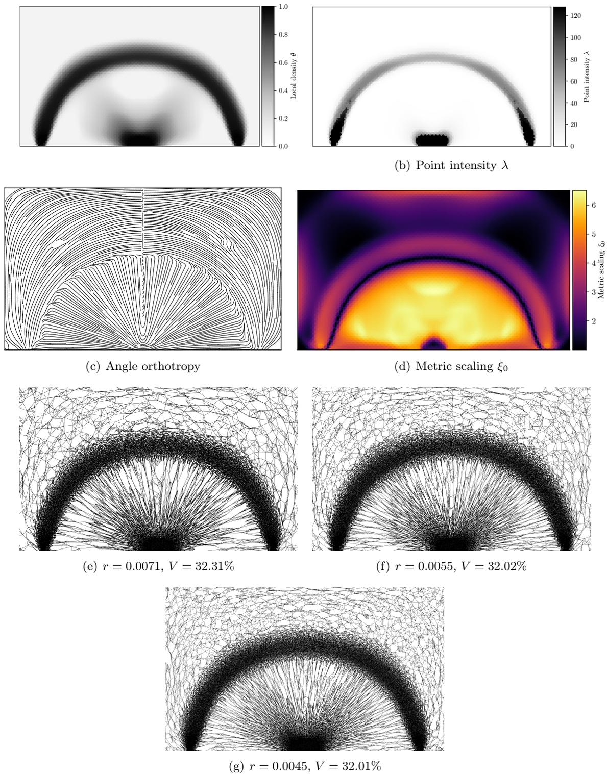
Figure 6.11: Orthotropic case. Volume constraint  $V = 30\%$ . Compliance  $J^*(p) = 60.2$ .
