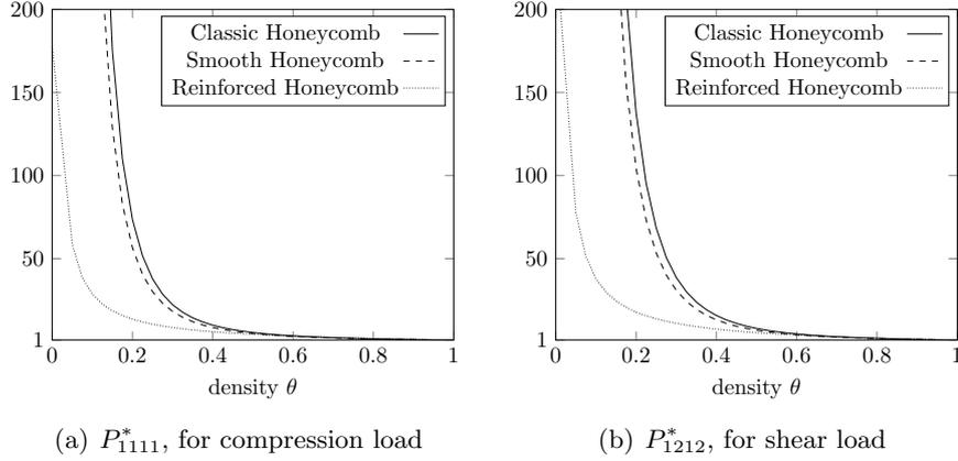
Figure 3.7:  $L^2$ - norm of the corrected stress depending on the density of the microstructures
