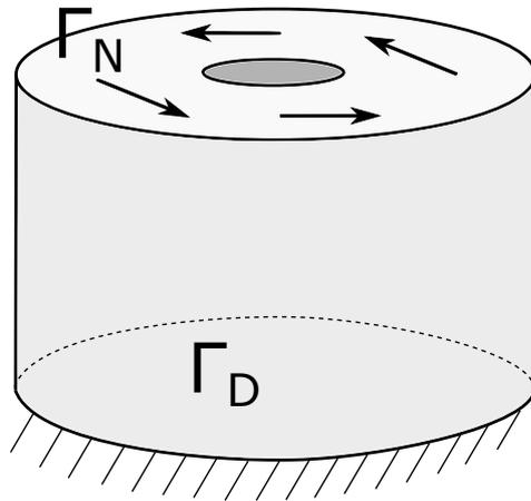
Figure C.4: Boundary conditions for the tube case
