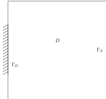
Figure 3.8: Boundary conditions for the cantilever problem
