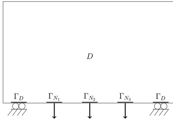
Figure 3.17: Boundary conditions for the gripping mechanism
