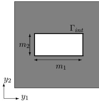
Figure 14: Example of parametrized periodic lattice material: a periodic square cell is perforated by a rectangular holes, whose length and height parametrize the geometry of the microstructure
