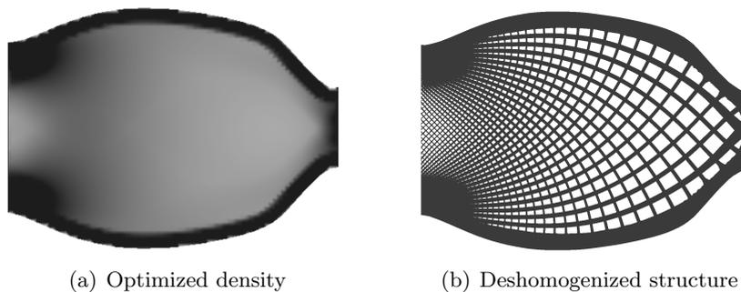
Figure 22: Results of topology optimization of a cantilever under a coating constraint by coupling homogenization and level-set methods
