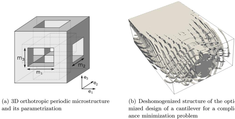
Figure 21: Projection (right) of a optimized design of a 3D cantilever for a compliance minimization problem (left)
