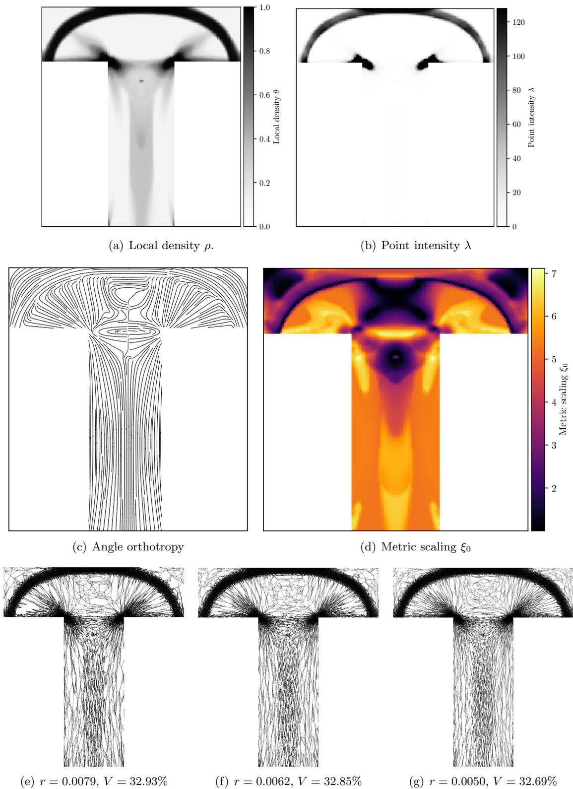
Figure 6.12: Orthotropic case. Volume constraint  $V = 30\%$ . Compliance  $J^*(p) = 65.1$ .
