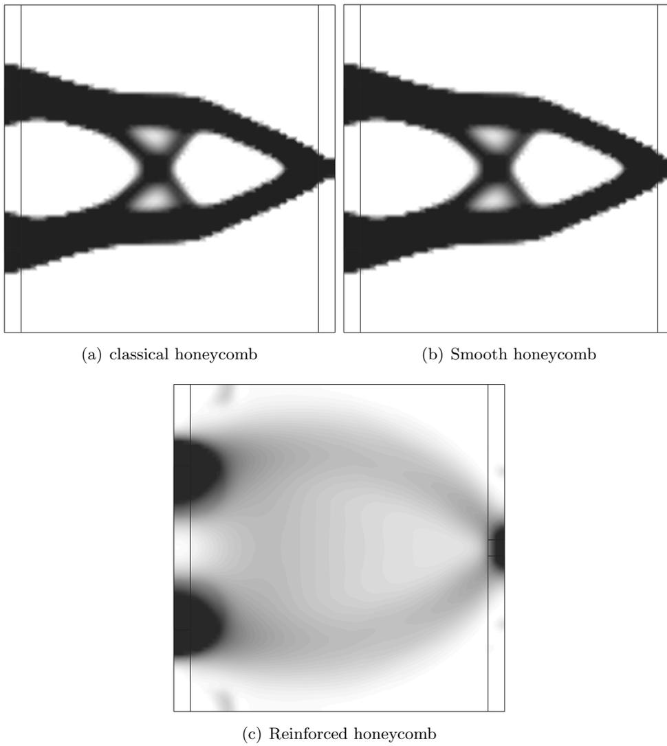
Figure 3.22: Optimized structures for the stress minimization
