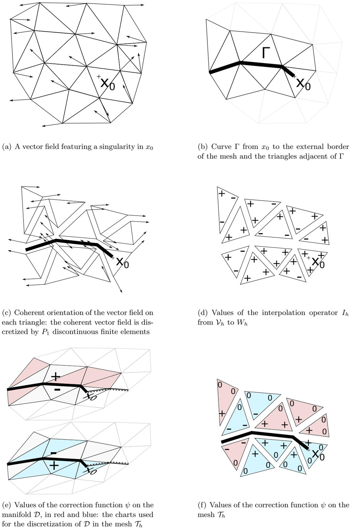
Figure 5.18: Numerical construction of a correction function
