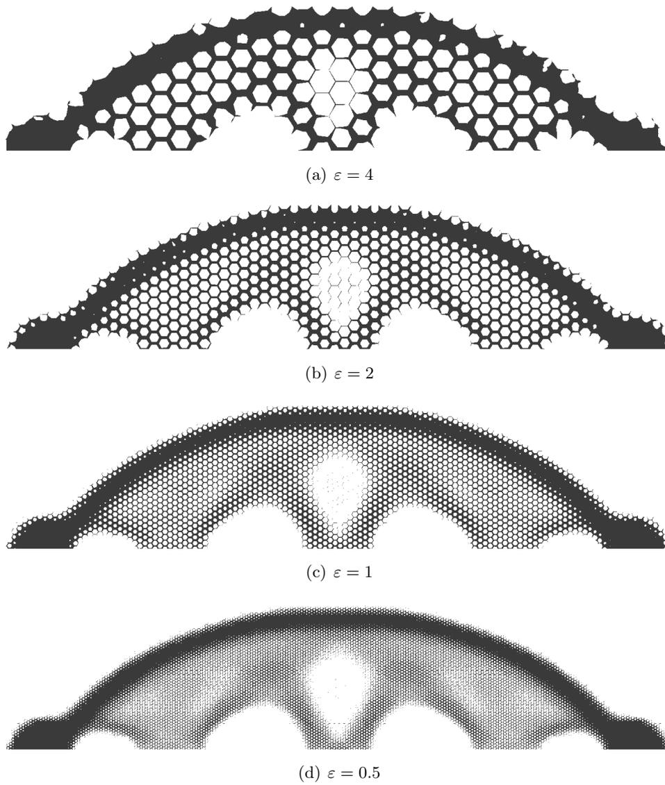
Figure 3.36: Projection of a radial density  $\theta$  over a classical honeycomb composite, for several sizes of cell  $\epsilon$
