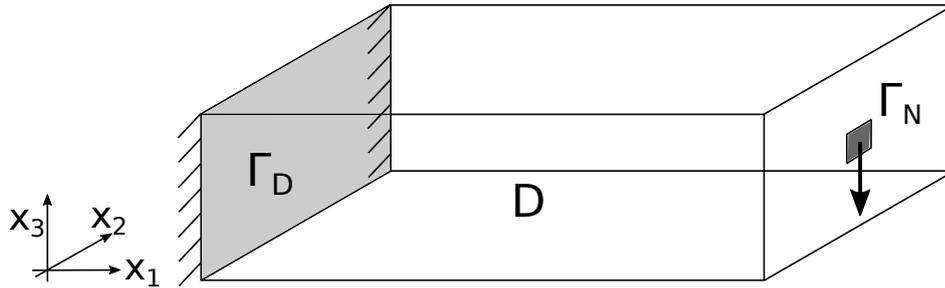
Figure 7.3: Boundary conditions for the cantilever problem
