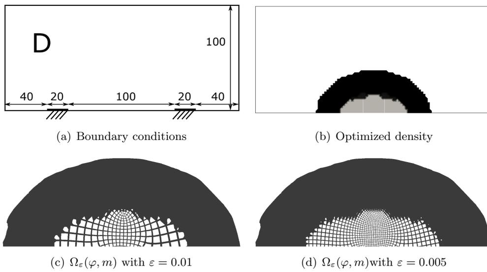
Figure 8.7: Numerical results in a design-dependent load case
