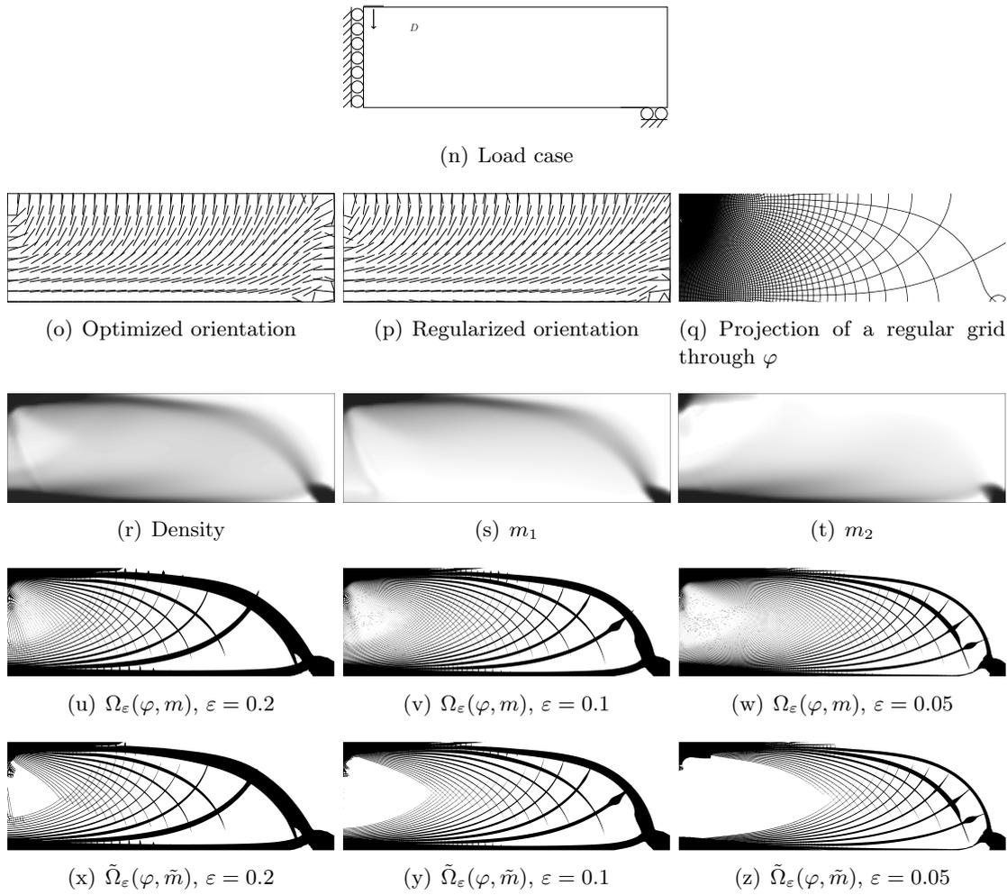
Figure 4.28: Complete process for a MBB beam
