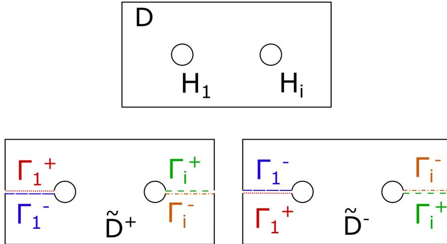
Figure 5.11: From a perforated domain  $D$  (top), a manifold  $\mathcal{D}$  is introduced. This manifold  $\mathcal{D}$  is cut along the curves  $\Gamma_i^\pm$ , this leads to two disconnected copies of the simply connected domain  $\tilde{D}$ . To find back the manifold, those copies have to be glued together along the cut lines  $\Gamma_i^\pm$  (the segments of the same color are connected in the manifold  $\mathcal{D}$ ).
