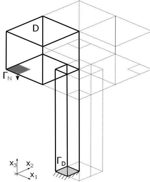
Figure 7.19: Boundary conditions for the bridge case
