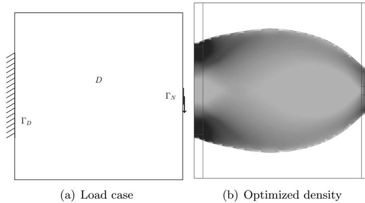
Figure 8.1: Cantilever test case
