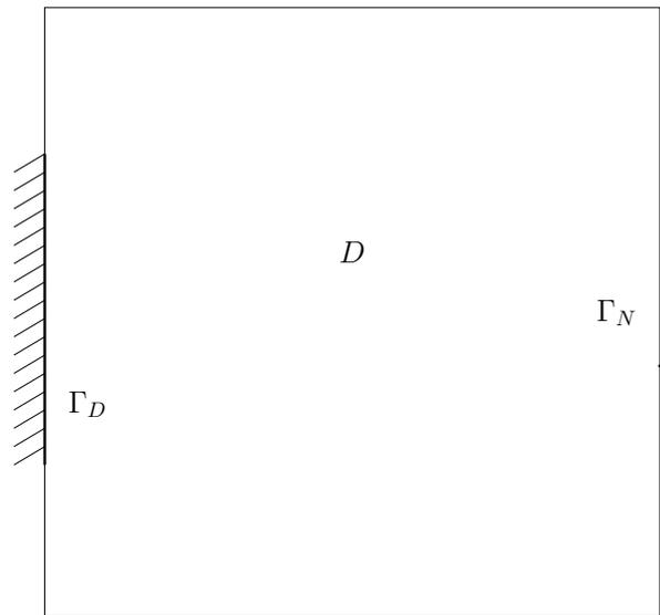
Figure 3.20: Boundary conditions for the stress minimization problem
