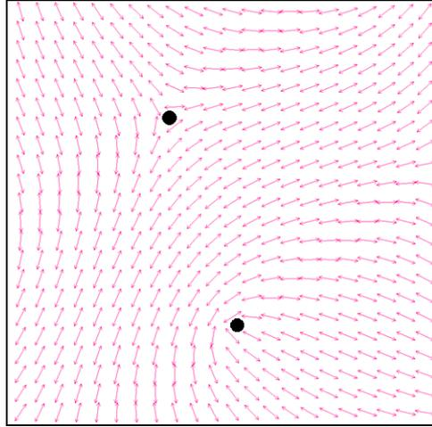
Figure 5.19: Direction field featuring two singularities (black points)
