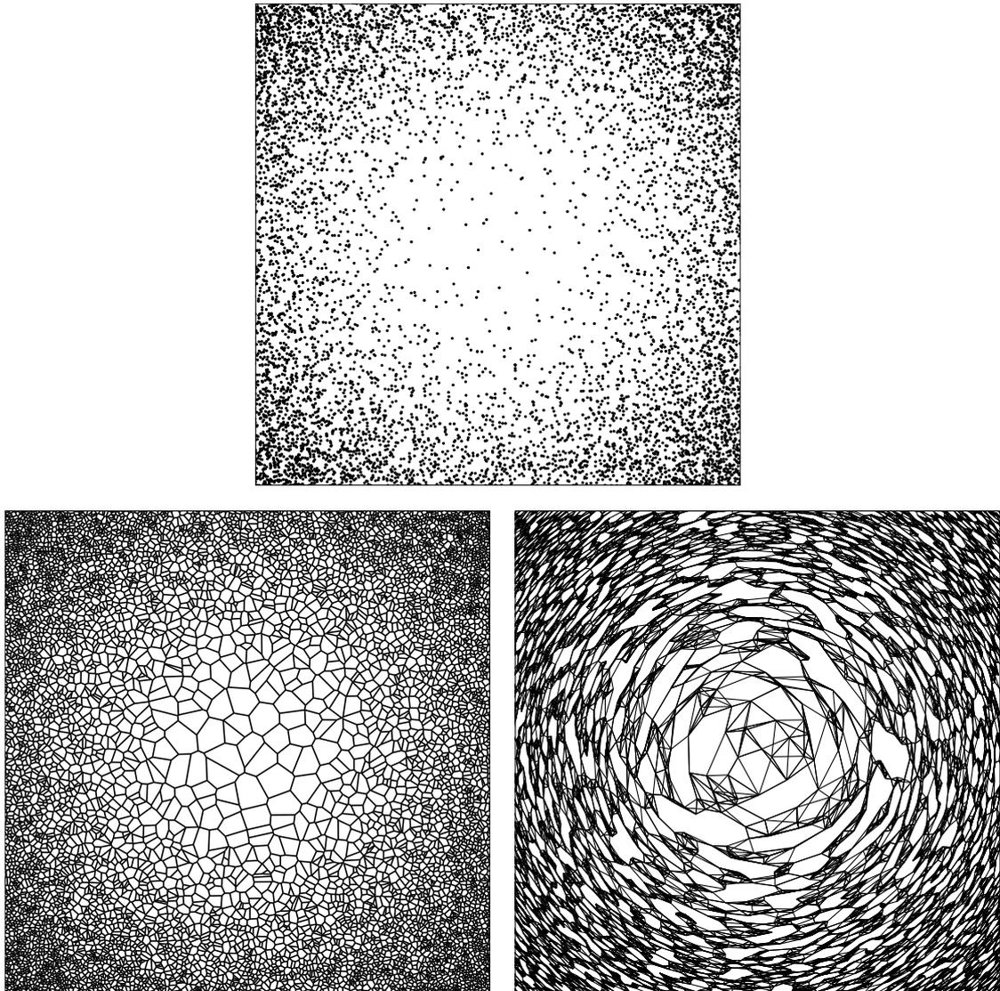
Figure 6.7: Grading material density with stochastic parametrized microstructures. **6.7(a)**: Inhomogeneous Poisson point process in the unit square with  $\lambda(\epsilon) = 500 \left(1 + 200 \|\epsilon - [0.5, 0.5]\|^3\right)$ . **6.7(b)**: Corresponding Voronoi microstructure. **6.7(c)**: Corresponding  $k$ -nearest microstructure with concentric variation of the metric rotation  $\theta$  and a constant metric scaling  $\xi = \{4, 1\}$ .
