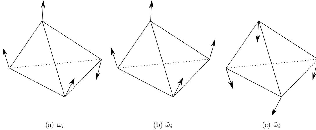
Figure 7.11: Optimized orientation field  $\omega_i$  (a) on a tetrahedron and the both possible coherent orientation fields  $\tilde{\omega}_i$  from  $\omega_i$  : the coherent orientation when the first vertex  $x_1$  is the upper one (b) and the coherent orientation when the first vertex  $x_1$  is the vertex on the right (c)
