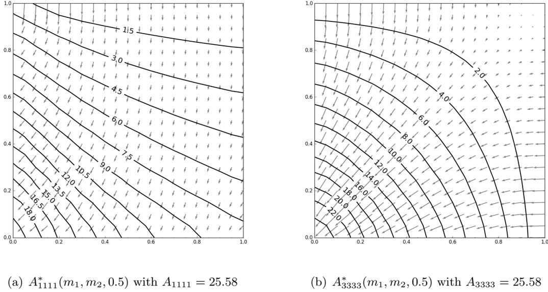
Figure 7.2: Isolines of the entries of the homogenized coefficients  $A_{1111}^*$  (left) and  $A_{3333}^*$  (right) and their gradients (small arrows) according to the parameters  $m$ , with  $m_3 = 0.5$ . The  $x$ -axis is  $m_1$ , the  $y$ -axis is  $m_2$
