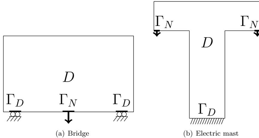
Figure 6.8: Boundary conditions for the bridge and the electric mast problems
