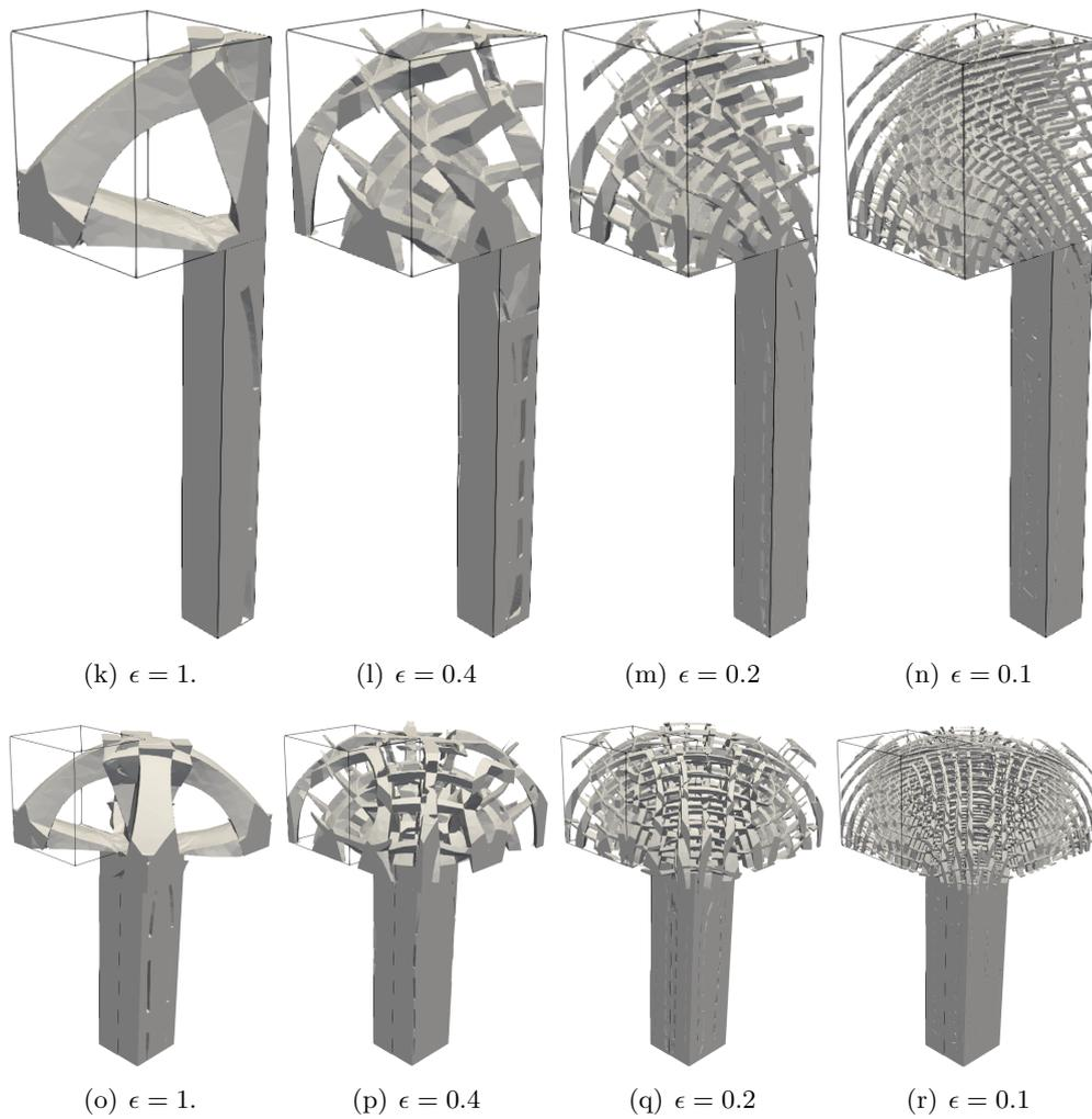
Figure 7.21:  $\Omega_\epsilon(\varphi, m)$  for several  $\epsilon$  in the electrical mast test case on the quarter of the whole domain (up), and on the whole domain (down).
