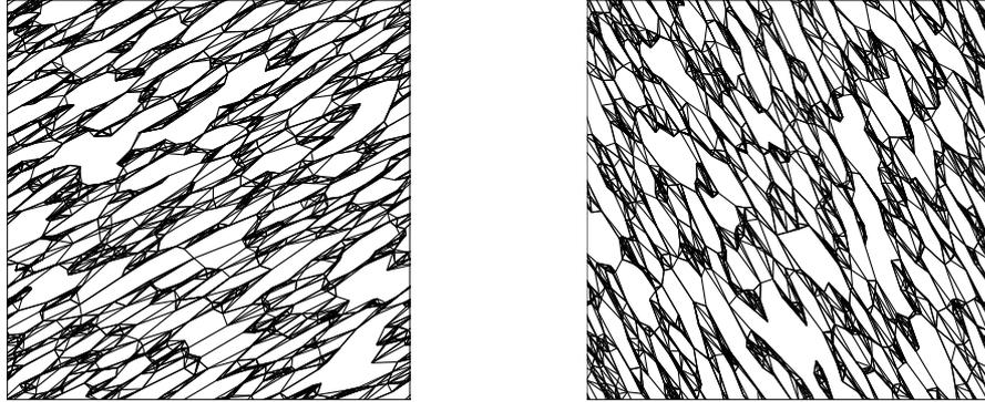
Figure 6.5: Two  $k$ -nearest graph microstructures induced by the set of points of Figure 6.2 (periodic domain), with  $k = 6$ ,  $r = 0.003$ , and  $\theta = R(30^\circ)$ .  $R$  corresponds to a two dimensional rotation matrix (counter-clockwise). 6.5(a): Metric scaling  $\xi = \{4, 1\}$ . 6.5(b): Metric scaling  $\xi = \{\frac{1}{4}, 1\}$ .
