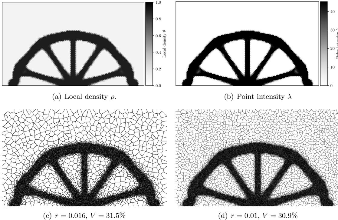
Figure 6.9: Isotropic case for the bridge. Volume constraint  $V = 30\%$ . Compliance  $J^*(p) = 63.8$ .
