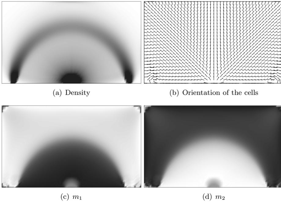
Figure 4.8: Optimized design of the bridge with rank-2 laminates
