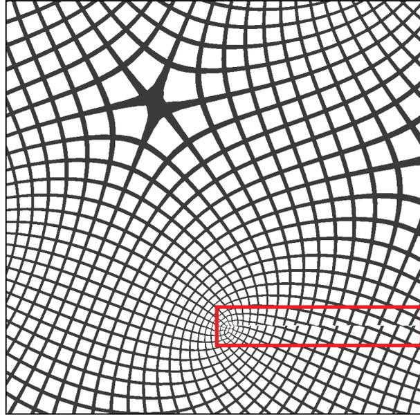
Figure 5.22: Projection of regular square cells according to the direction field  $\alpha$  defined on  $D = [0.5; 2] \times [0.25; 1.75]$  with non integer coefficients : failures in the connectivity between the bars along  $\Gamma_i$  (in the red rectangle)
