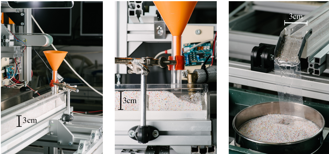
Figure 2.3 – Details of the flume experiment. Left. Flume inlet. Grains delivered by the sediment feeder fall into a funnel which directs them into the channel. Center. Detail of the flume inlet. Sediment grains fall from the funnel. They initially stay at the surface of the flow, and gradually settle on the bed. They are then entrained by the flow as bedload. Right. Flume outlet. Grains are separated from the fluid by a sieve. The funnel diameter is 10 cm and the flume width is 3 cm.
