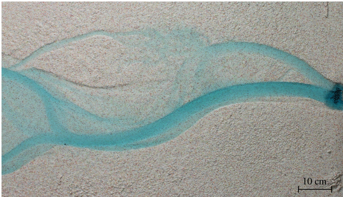
Figure 3.15 – Planform geometry of a braided laboratory river. Input parameters: Q_w = 1.0 \text{ L/min} and Q_s = 1.7 \text{ g/min} .
