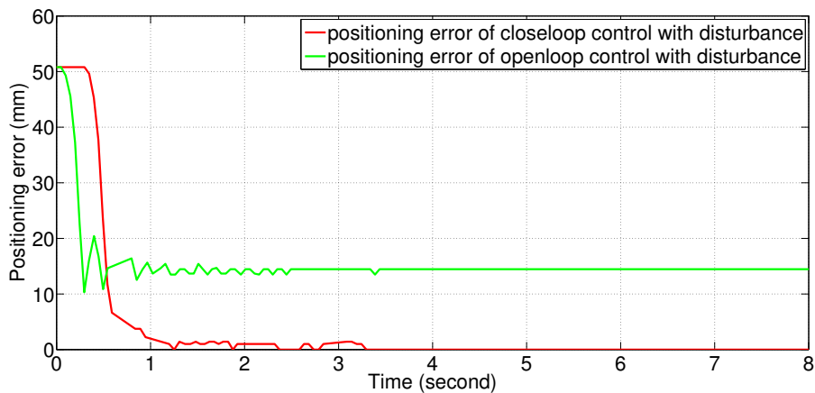
Figure 3.8: Comparison of positioning errors between open-loop control and closed-loop control with unknown disturbance
