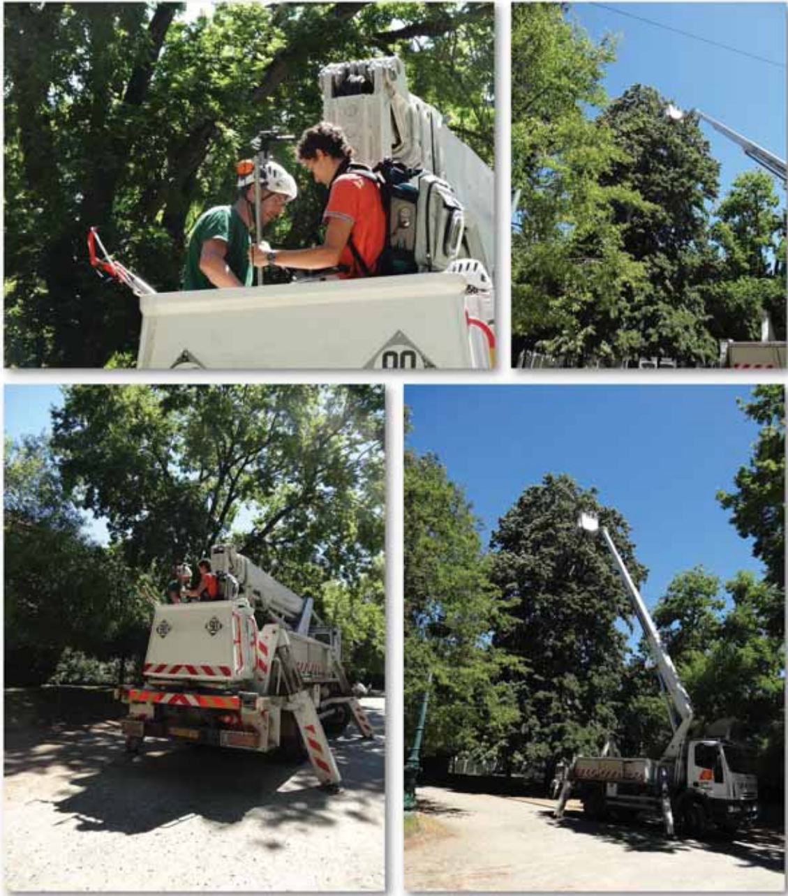
Figure 3.20: Illustration of the canopy level spectral measurements carried out thanks to a cherry picker of Toulouse city.
