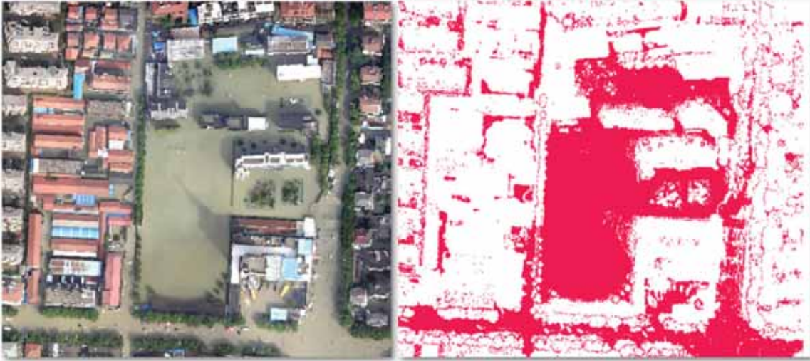
Figure A.2: Flood mapping results obtained in the work of (Feng et al., 2015). Left: study site with visible inundated areas. Right: resulting map with the detected inundated areas colored in red.
