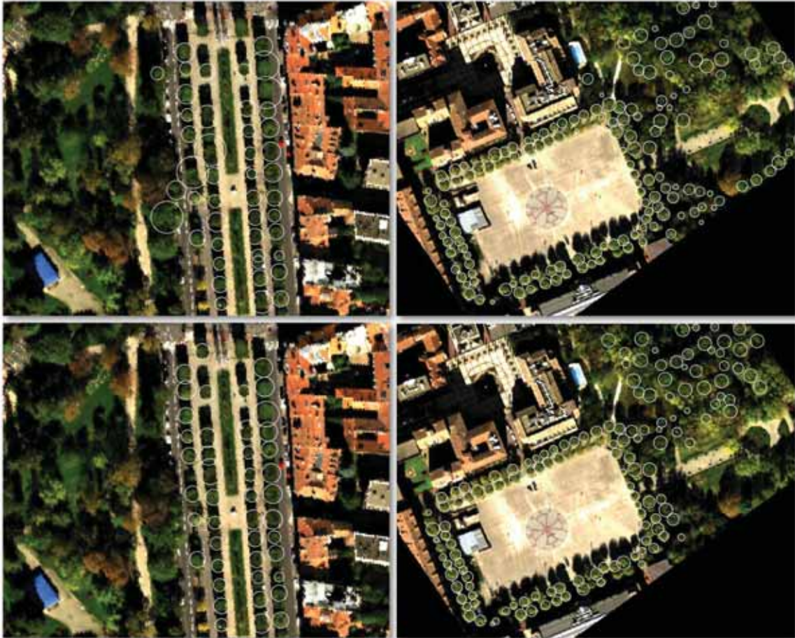
Figure 3.25: Top: without GIS and without the height. Bottom: without GIS and without the angle. Left: first study site. Right: second study site.
