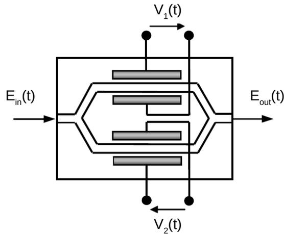
Figure 4.3: Simplified diagram of a dual-drive Mach-Zehnder modulator
