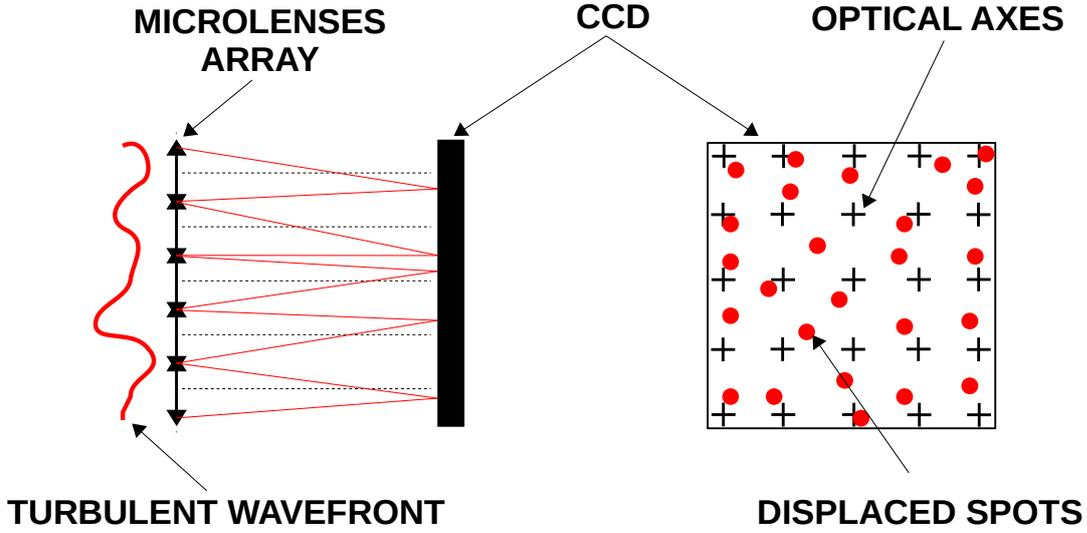
Figure 3.2: Schematic diagram of the Shack-Hartmann analyzer
