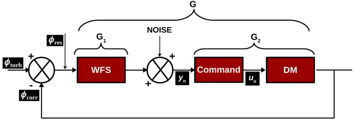
Figure 3.3: Simplified diagram of the servo-loop of an AO system. The transfer functions detailed in 3.2.1.4 are reported. The wavefront analyzer is downstream of the DM, therefore it measures a residual wavefront. Note that the noise is in fact neglected in the subsequent developments as explained in 3.2.1.1.2.
