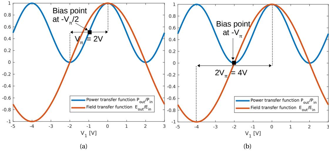
Figure 4.4: Mach-Zehnder transfer function for intensity (blue) and field (orange). (A) Bias point and peak-to-peak voltage sing required for OOK modulation. (B) Bias point and peak-to-peak voltage sing required for DBPSK modulation.
