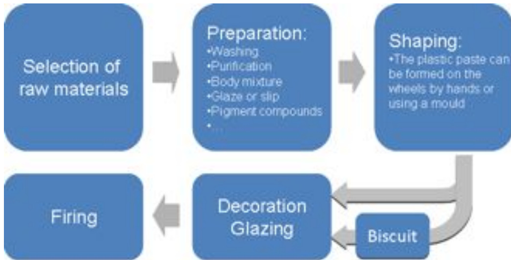
Figure 1.4 The flow diagram of the manufacturing process of ceramics.
