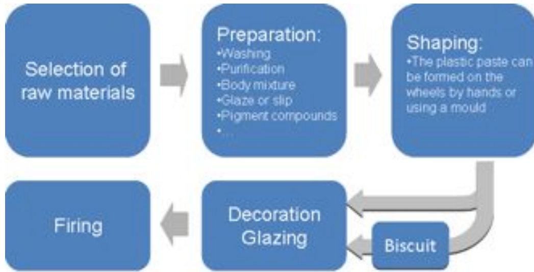
Figure 1.4 The flow diagram of the manufacturing process of ceramics.
