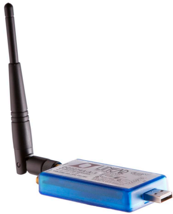
(a) DC2274: Low-power wireless manager (1 deployed)
