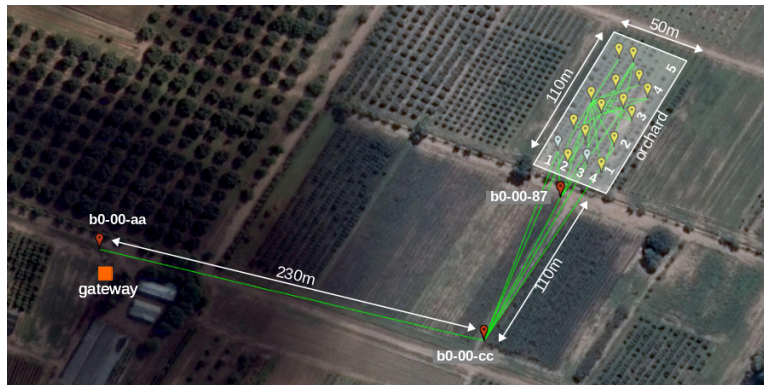
Figure 4.7: Areal view of the sensor network deployed in the orchard near Mendoza, Argentina.
