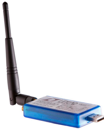
(a) DC2274: Low-power wireless manager (1 deployed)
